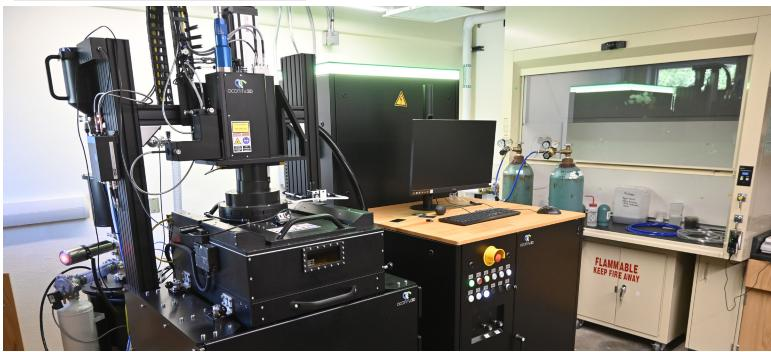
Sounds cool, doesn't it? Or at least, pretty complicated. Abbreviated LPBF, this process is used by specialized devices to create materials like a 3D printer, melting alloy powders into solid products, layer after layer. The Materials Engineering Department recently acquired one of these devices for around \$500,000; a half a million dollars. As I am a Materials student myself, I had a direct connection to talk to Dr. Majumdar, the man who secured the device, about its functionality and purpose.
