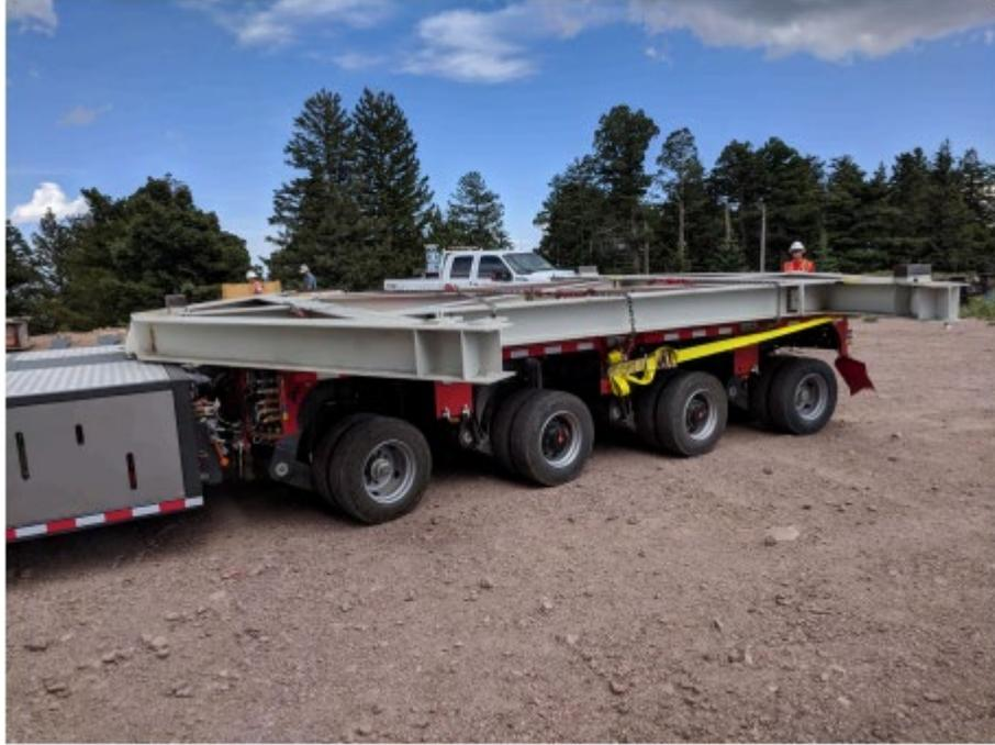
Figure 2: Assembly jig installed on the transporter.
