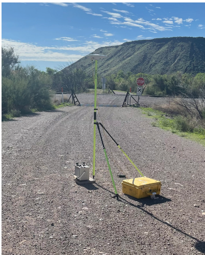
FIGURE 6. Instrument setup used during the survey, with the gravimeter (small gray box on the left of the paver) pointing to the north and the GPS system planted on the southwest corner. Mesa del Contadero is on the right. To the left of the mesa is the site of the 1862 Battle of Valverde, the largest Civil War battle in the western United States (Koning, this volume).
