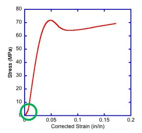
The circled part is the "start-up toe" which results from the sample not being exactly a right cylinder. It usually extends to a strain of about 0.005. For a 1 in sample, this is 0.005 in ~0.1 mm which is a reasonably small sample prep tolerance. It is assumed that the initial part is linear and that it follows the linear behavior that extends out to 0.03 or so.
