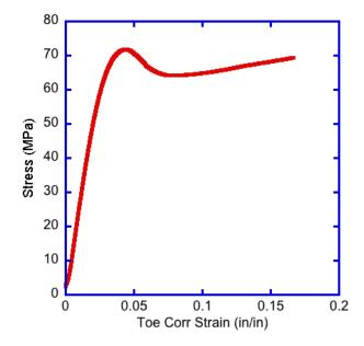
5) Since the cross-sectional area increases as the sample is compressed approximately so that the volume is constant, the true stress = Force/A=StressEng\*A0/A where A is the true area and A0 is the initial area. Volume=A0\*L0=A\*L -> A0/A=L/L0=(L0- $\Delta$ L)/L0=1-StrainEng
