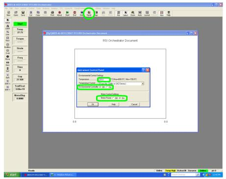
Clicking "Panel" will bring up the Instrument Control Panel which can then be used to toggle the motor and environmental chamber on/off as well as set the temperature of the environmental chamber. It is imperative that the fixtures be free of samples/obstructions when the motor is turned on to avoid damage to the instrument.
