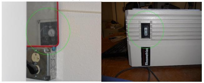
The switch tends to stick in the half on position, to ensure the software and the system sync correctly, the switch must be turned on in one swift motion.
