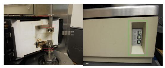
The red lines on the leftmost photo show potential impact points. Do not crash the enviornemental chamber into the fixtures as it will destroy the machine. Use the buttons indicated on the right to adjust the fixture to the correct height. These buttons move the upper fixture the direction indicated. Pressing the middle button in conjuction with one of the other buttons accelerates the movement of the fixture greatly.
