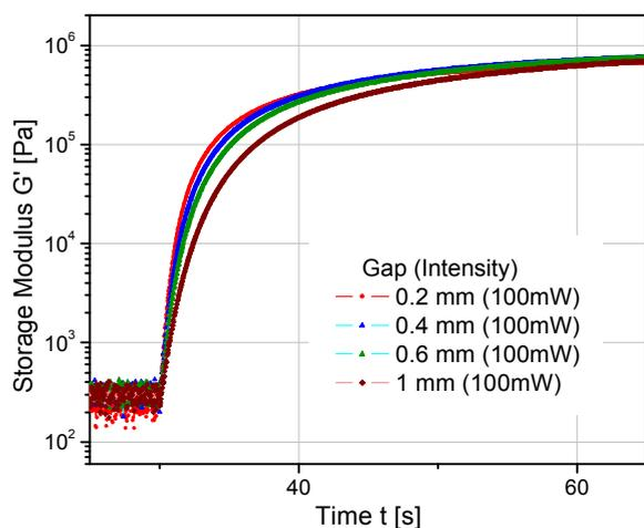
Figure 4: Effect of sample gap to the UV curing reaction
