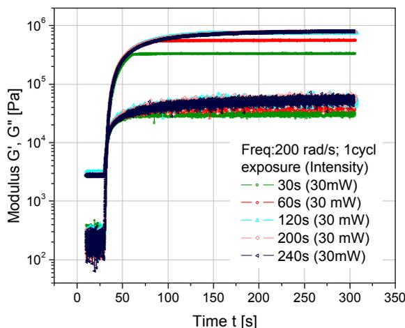
Figure 7: UV-initiated curing under 30mW intensity and different exposure time
