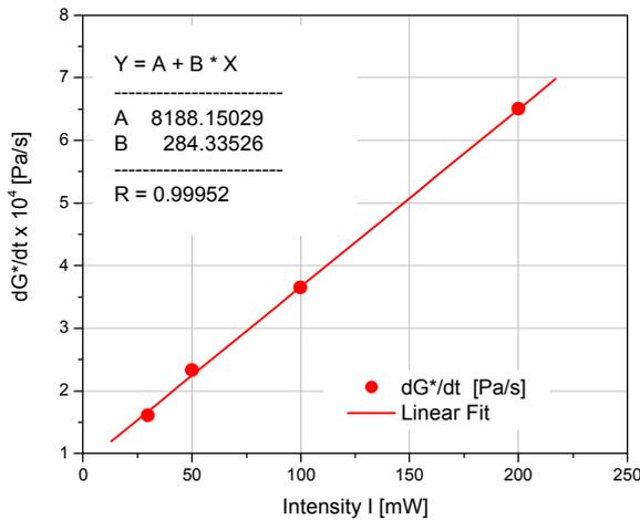
Figure 6: The reaction rate ( $dG^*/dt$ ) vs UV exposure intensity
