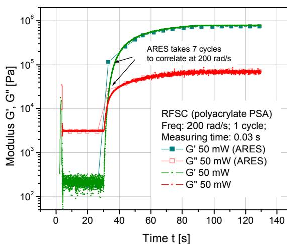
Figure 3: Monitor of UV-curing reaction on ARES LS2 rheometer. Data collected by ARES rheometer and fast sampling acquisition
