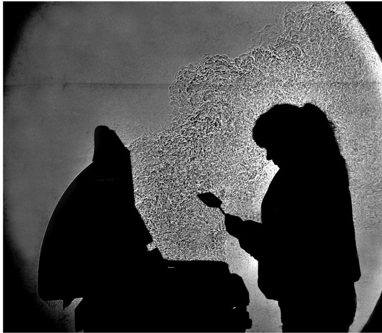
**Figure 13.** Large-scale retroreflective shadowgram showing thermal effluent from outdoor cooking on a grill, reproduced with permission from FloViz Inc.
