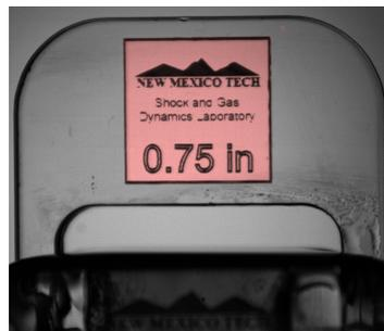
**Figure 5.** A representative image taken of the focusing plate before testing. The pixel area within the outer square is measured by a MATLAB script and represented by the red region shown.
