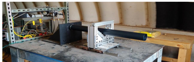
Figure 2: Thrust test stand with motor case inserted. Nozzle and force transducer assembly not pictured.
