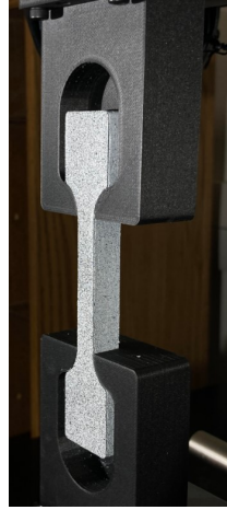
Figure 5.7: JANNAF tensile sample positioned within the tensile heads printed using a Markforged 3D printed using Onyx with fiberglass reinforcement.
