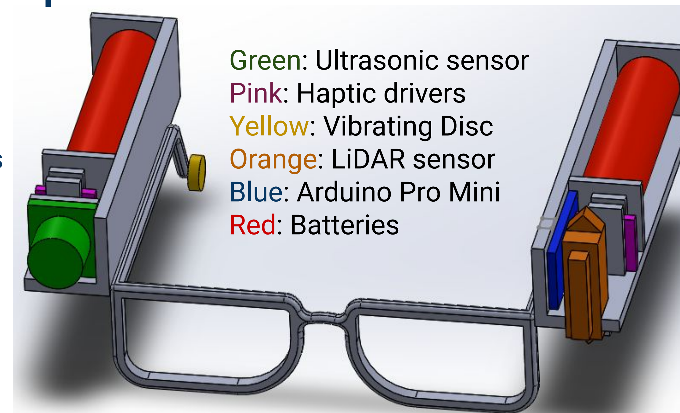
Figure 3: CAD model of prototype and electronics
