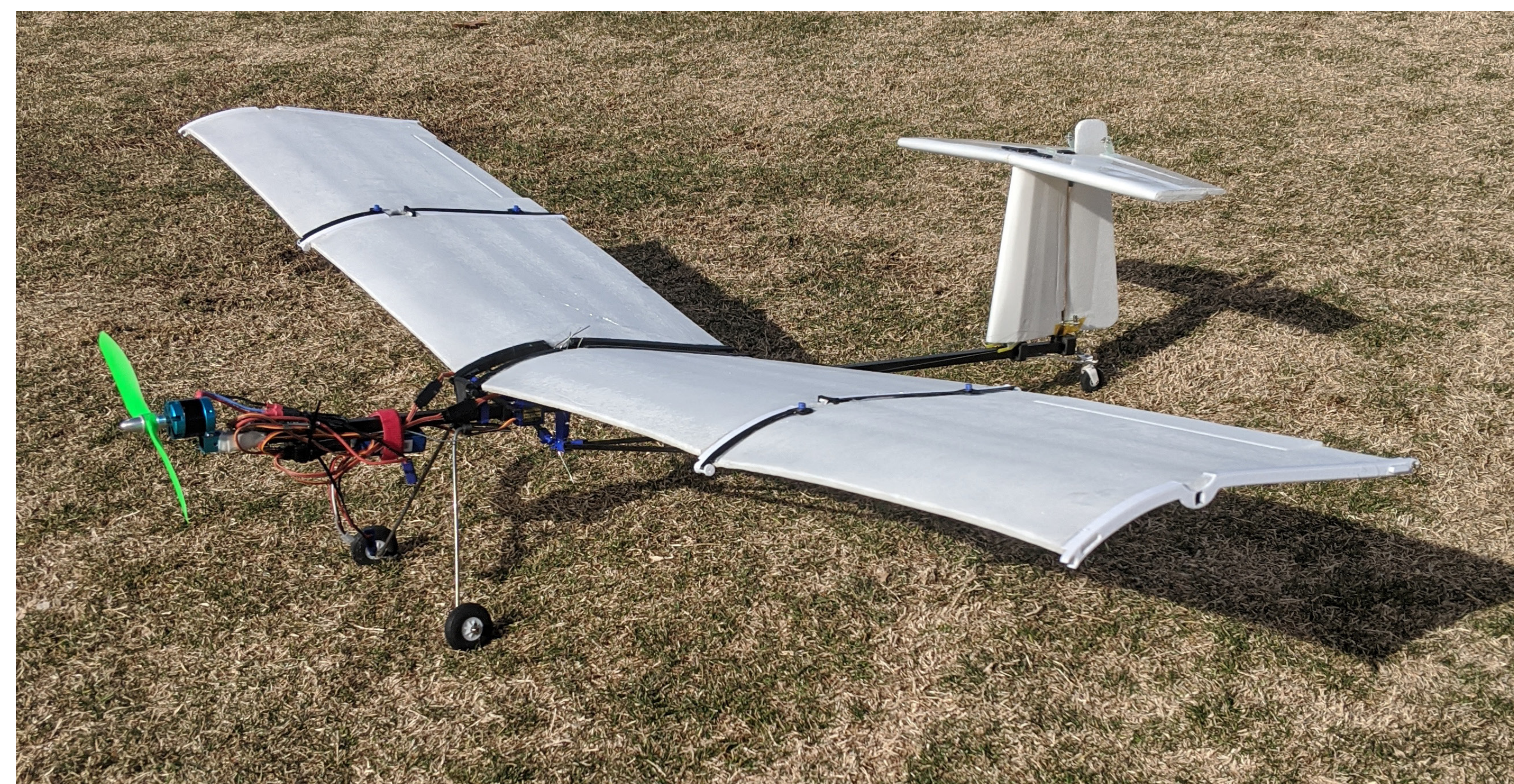
Our final aircraft design during testing without the payload installed
