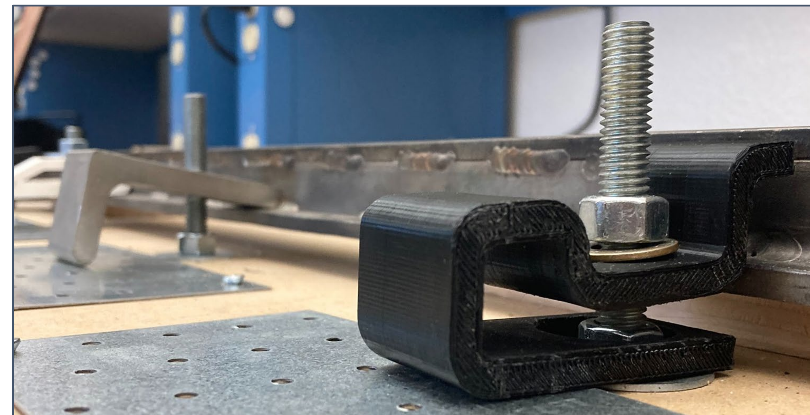
Figure 2. 3D Printed Lug in physical testing setup.
