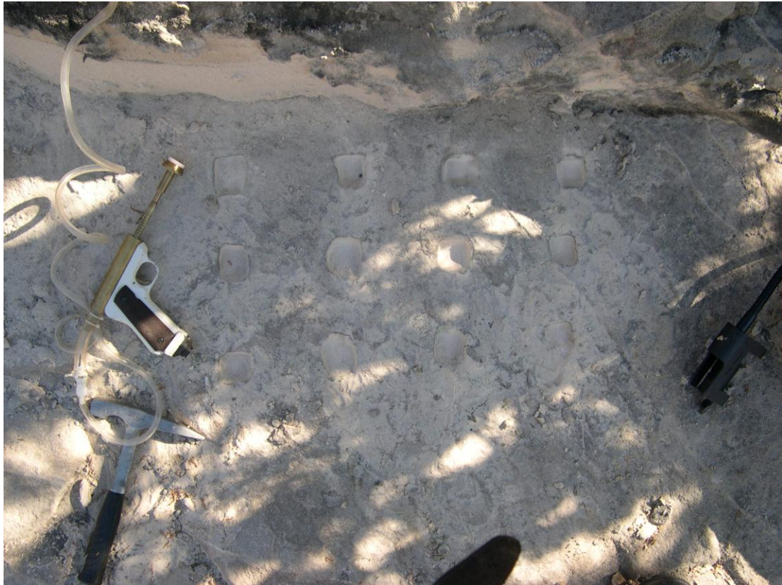
Figure 6. Outcrop photo of prepared site for field permeametry. Note prepared 4X3 sampling grid and field permeametry gun. Rock hammer for scale. From Navajo Sandstone at I-70 site.
