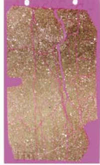
M1 UK-2056.16 Notch indicates natural fracture with dip of ~11- 15°
