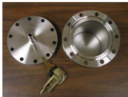
Fig. 6. Photographs of canisters built from high vacuum equipment to preserve noble gases that will degas from pore fluids in core samples.
