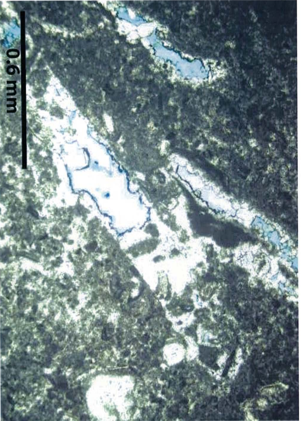
Figure 23 Photomicrograph of a biomicrorite. Sample shown has had some pore space occluded by calcite crystals. A large recrystallized phylloid algal blade is present in the center of the thin-section. The dark material in the thin-section is mostly micrite with a few fossil fragments. The blue indicates porosity.
