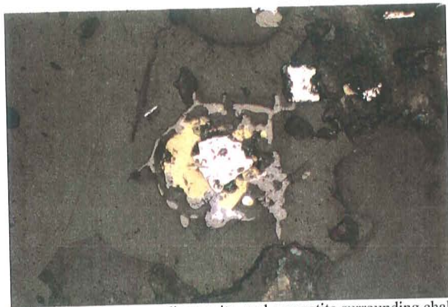
Photo 16: Chalcopyrite surrounding pyrite, and magnetite surrounding chalcopyrite, sample SD-23-1556 ft. (f.o.v. = 0.45 mm long).
