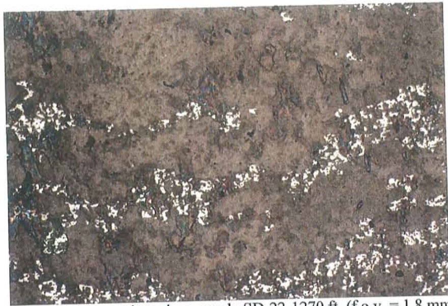
Photo 6: Parallel magnetite veins, sample SD-22-1270 ft. (f.o.v. = 1.8 mm long).
