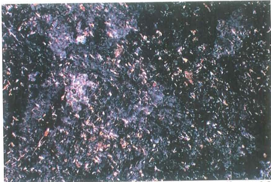
Photo A.22: Fine grain white phyllosilicates altering plagioclase (f.o.v. = 0.9 mm long). Sample SD-16-2629 ft.
