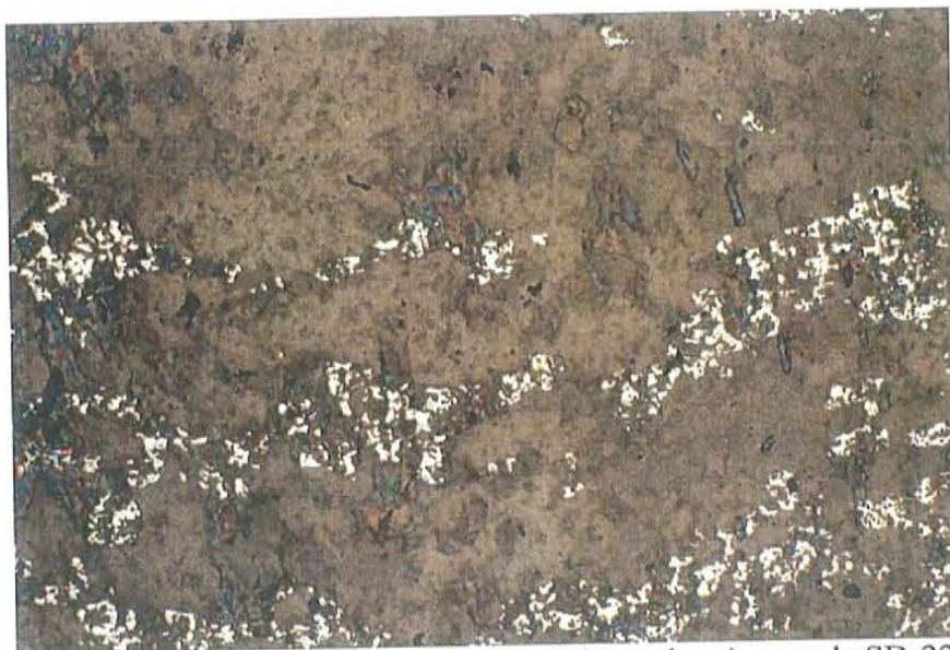
Photo A.47: Parallel magnetite veins (f.o.v. = 1.8 mm long), sample SD-22-1270 ft.
