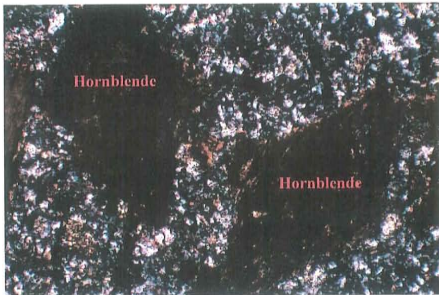
Photo A.38: Hornblende altered to smectite (f.o.v. = 0.9 mm long), sample SD-21-1852.5 ft.
