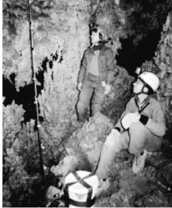
Figure 8.23: The Tray Room in Torgac Cave, NM. Kaolinite clay samples were suspended at 30 cm intervals to monitor vertical variations in relative humidity [Forbes, 1998].
