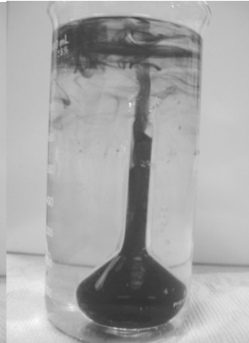
Figure 6.40: Density driven flow. Water temperatures in the container and in the flask are 17.6°C and 33.1°C, respectively. Vigorous water exchange takes place.
