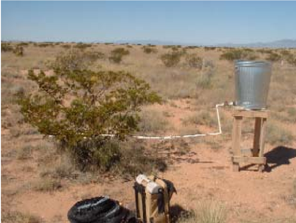
Figure 2-5: Irrigated Shrub and Irrigation system. The spectroradiometer is visible in foreground
