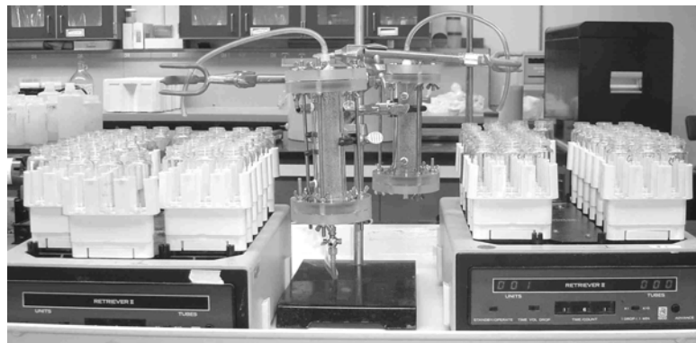
Appendix Figure D-2. Laboratory setup for column experiments.
