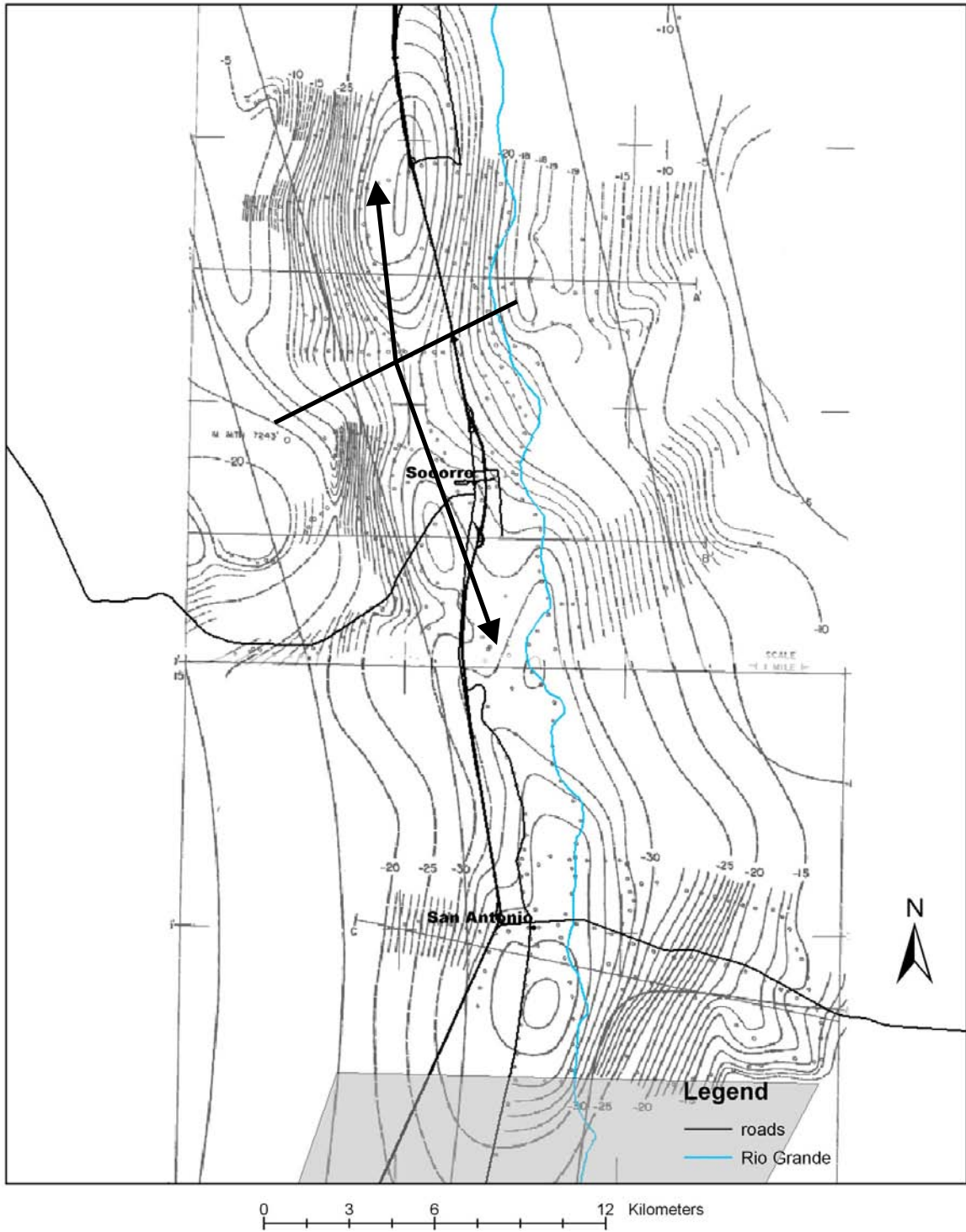
Figure 48 Inferred location of anticline according to residual Bouguer anomaly map (Sanford, 1968). Arrows denote limbs of anticline.
