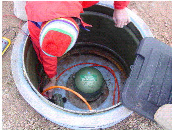
Figure 3.6: Centering of an STS-2 inside a completed vault just prior to capping. The three pendulum masses are centered by pushing a button on the small green box shown (manipulated in the photo by PASSCAL's Tim Parker), and then verifying that the mass-position voltages read off the Flukemeter are within 2 V of zero. The orange cable shown is wrapped around the sensor once completely and then secured onto the blue foam insulation at two points opposite each other to reduce the coupling of noise to the STS-2 when the cable is subject to thermal variations. (Photo courtesy of Dan Klingsmith.)
