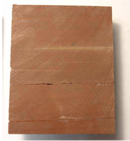
Figure 6.26: Large numbers of extension fractures are observed parallel to bedding and sub-parallel to the fluid pressure gradient. Thin section analysis will be used to quantify the number of fractures in the future.
