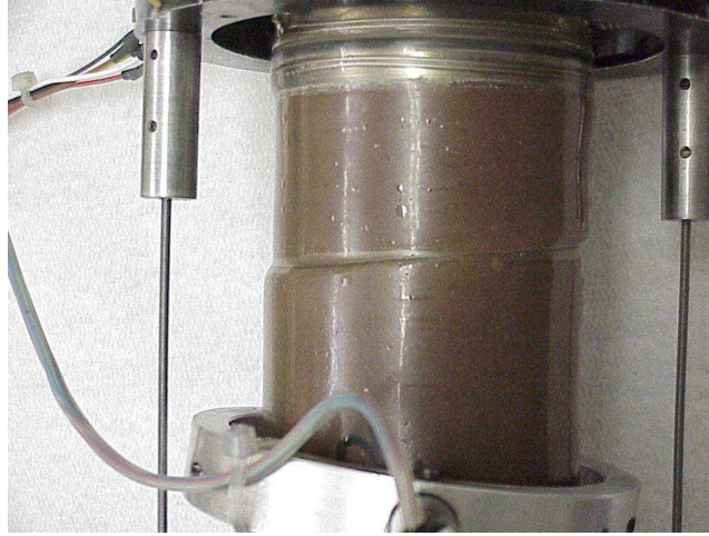
Figure 6.24: Generation of a shear fracture along a pre-existing extension fracture is the result of the angle of the extension fracture. The slip on the fracture is limited by the amount of stretching in the jacket of the specimen.
