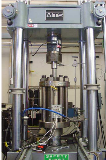
Figure 6.20: Pressure vessel and load frame used for generating hydraulic fractures. Tubing on right hand side allows for the simultaneous dropping of fluid pressure at top and bottom end caps.
