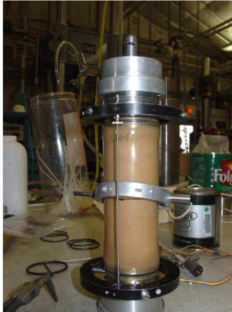
Figure 6.19: The endcaps used in the extension tests are able to support differential stresses, such that the maximum stress is the confining stress. Total assembly height is approximately 20 inches tall.
