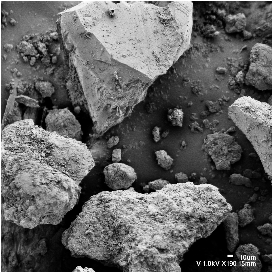
Appendix Figure B-5. SEM image of virgin SMZ (190X). Large particle in upper-center is quartz.
