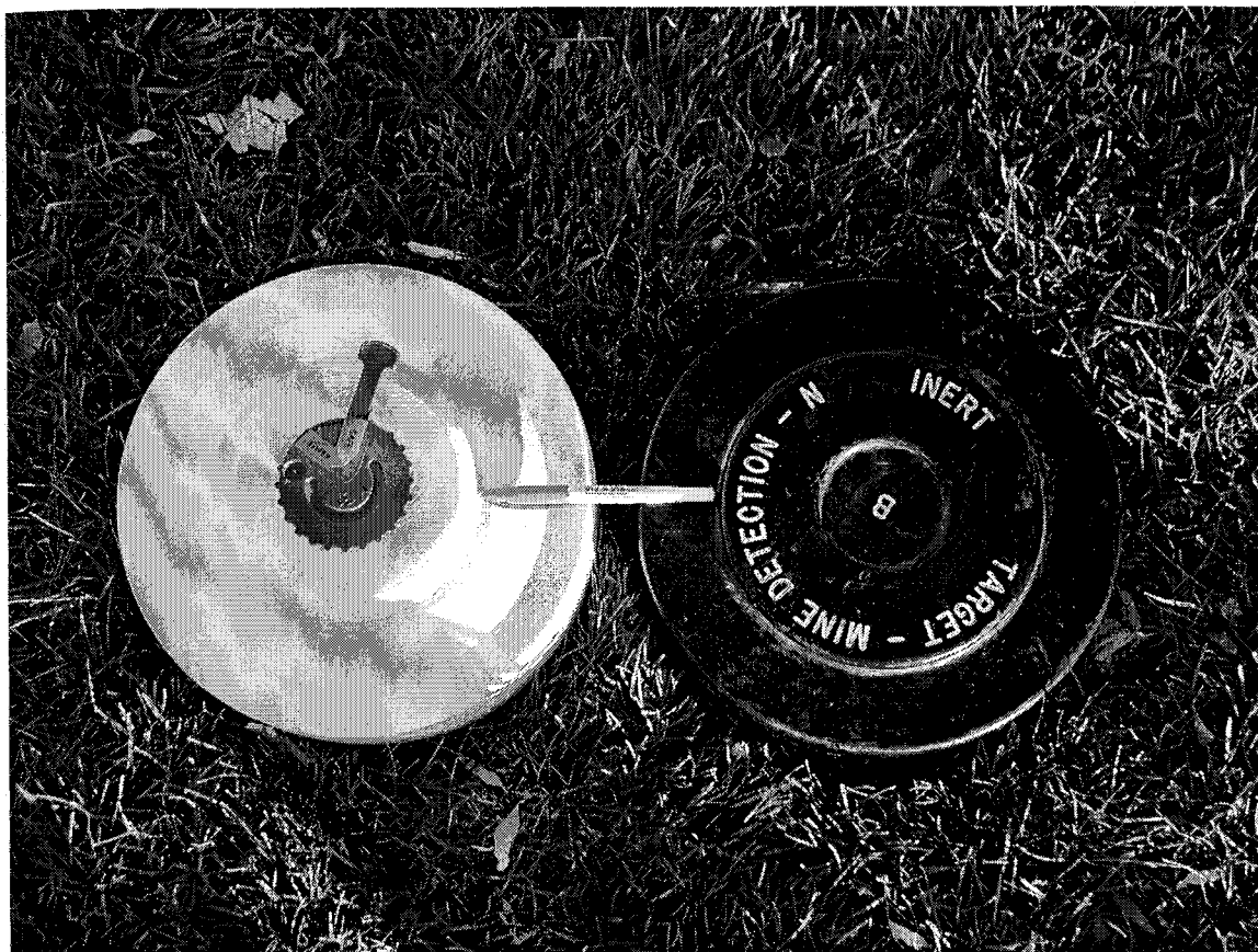
Figure 3.4 Netherland type NR26 simulant landmine (left) and U.S. Army edition inert target landmine (right).
