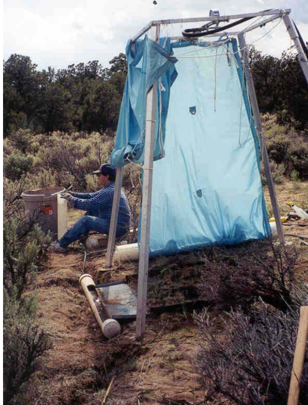
Figure 10: Sprinkler system over rainfall simulation plots. Tower height is 2.06 m.
