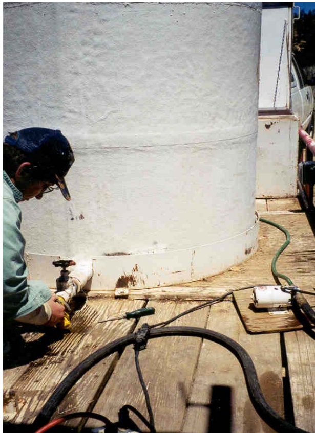
Figure 11: Original (above) and final set-up (below). The large pump was replaced by a small aquarium pump that delivered water to the sprinkler system.
