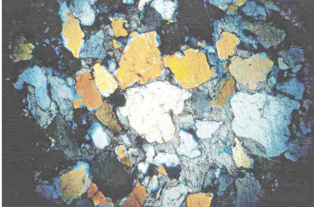
Figure A 1-6: Quartzarenite. Partial/total dissolution of feldspar produced pore spaces. These pore spaces were filled by calcite. Reid State B No1. 10914.7 ft-10915.6 ft. LA (Long Axis) =3.77mm
