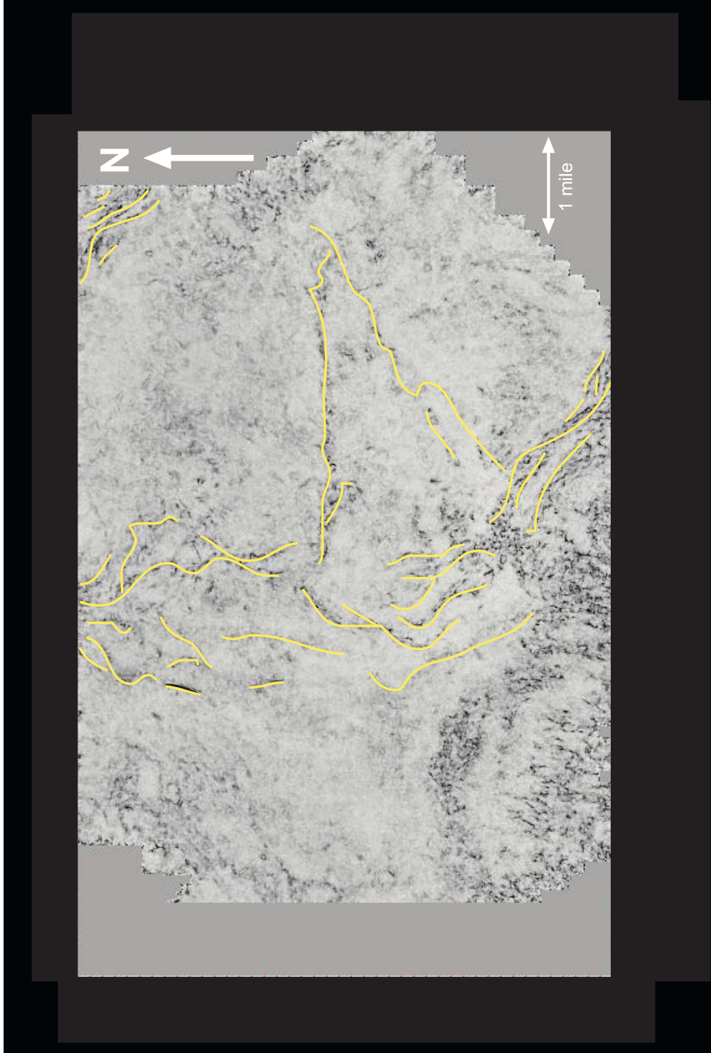
Figure 7.10: Fault recognition on the coherence analysis map, larger area of study. Yellow lines indicate major faults.
