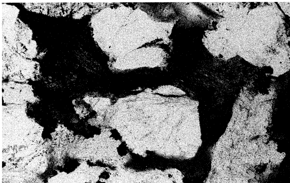
Figure 4.19 Photomicrograph of quartz grains surrounding a pore occluding, iron oxide replaced, fine-grained silicic lithic. Dissolution has occurred within the replaced, hematitic matrix and at the grain's margins. Hematite has also precipitated within fractures in several quartz grains. Compaction and the precipitation of authigenic cements, such as authigenic hematite, are responsible for the majority of diagenetically induced pore occlusion in this sandstone (image width = 1.3 mm).
