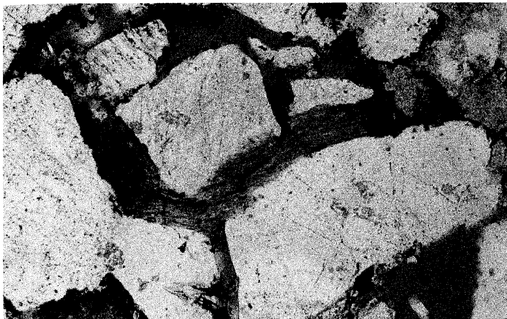
Figure 4.18 Photomicrograph exhibiting the compaction of a fine-grained, undifferentiated silicic lithic grain composed of hematite, kaolinite and potassic and sodic aluminosilicate minerals. Framework quartz grains and a smaller microcline grain have enclosed this ductile grain (image width = 1.3 mm).
