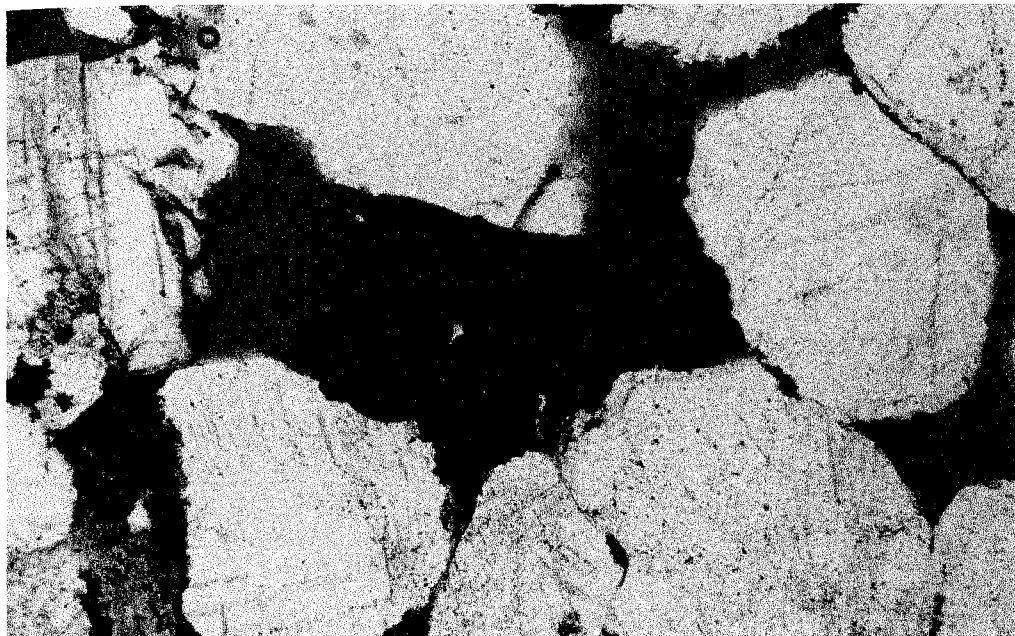
Figure 4.21 Photomicrograph of pore filling, authigenically precipitated and replaced ferroan cements (primarily authigenic hematite and ferroan dolomite clusters; image width = 1.3 mm).
