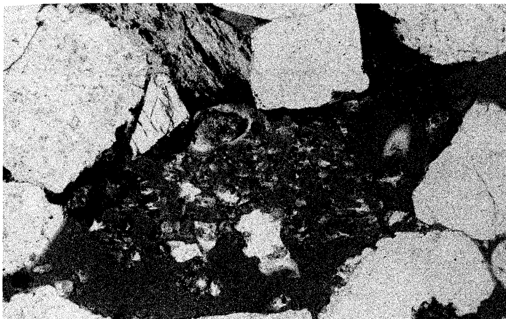
Figure 4.37 Photomicrograph showing late stage, secondary macroporosity created by the almost complete dissolution of a feldspar grain. Observe the large, euhedral, authigenic quartz overgrowths rimming the margins of framework grains in the lower left and middle right of the image. Authigenic quartz appears to be a more important diagenetic phase than modal analysis indicates (image width = 1.3 mm).
