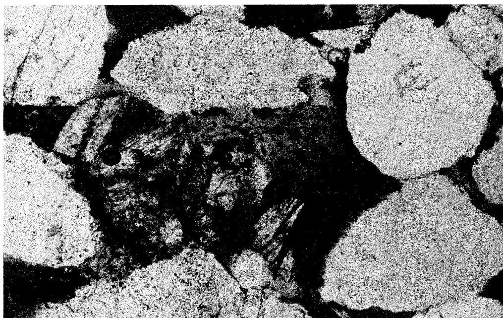
Figure 4.33 Photomicrograph of a partially dissolved feldspar grain and intragranular microporosity in authigenic kaolinite and potassic aluminosilicates. Whole and partially dissolved ferroan dolomite rhombohedral clusters occlude pore pathways, reducing the effective porosity of the sandstone (image width = 1.3 mm).
