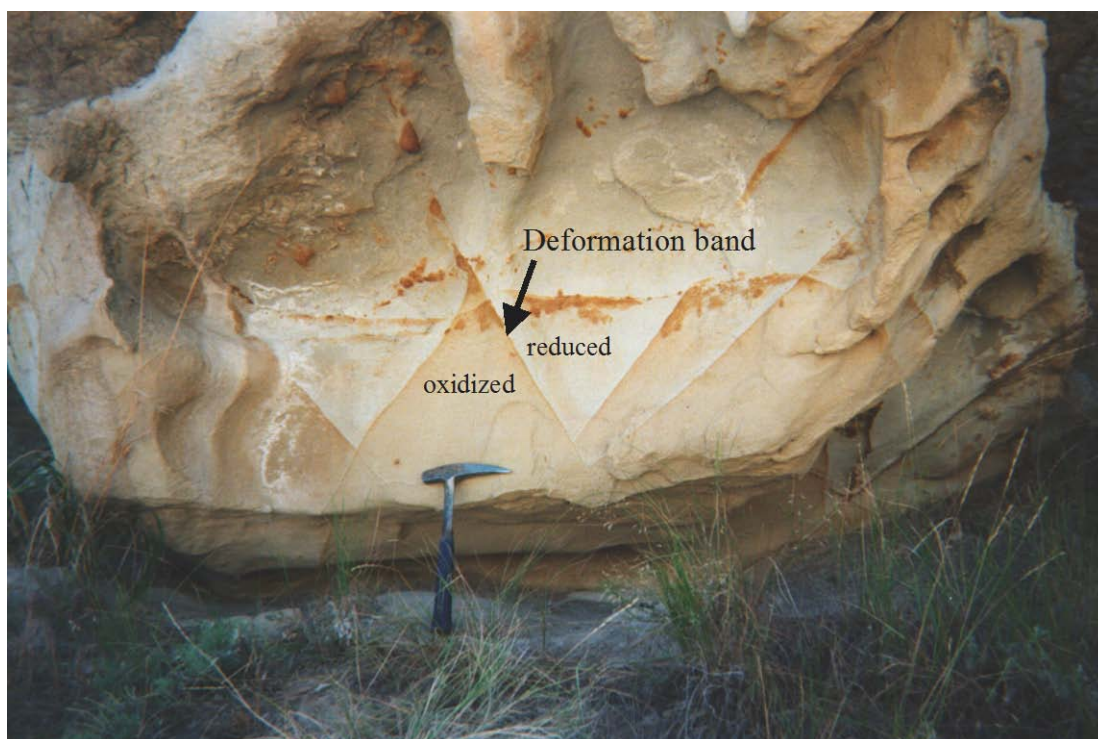
Figure 1-13: Conjugate deformation bands with a vertical bisector to the acute angle. Note reduced iron above the deformation bands and oxidized iron below.
