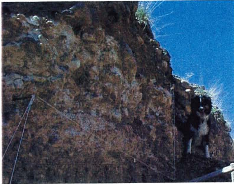
Figure 3.5. Picture of trench showing the stage III carbonate of the footwall, ~2 meters west of the fault plane. String lengths are a meter from nail to nail.
