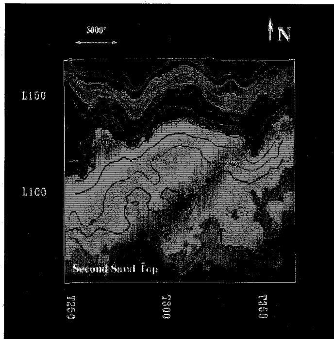
Figure 4.17: Time-structure map of the top of the Second Sand. Note the continued prominence of the central re-entrant in the upper slope.
