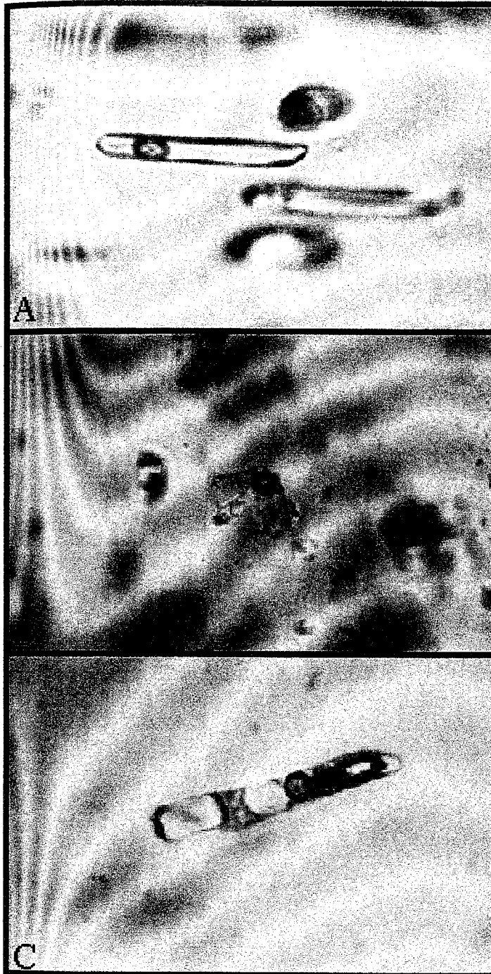
Figure 2 Photomicrographs of fluid inclusions in quartz to show the variation in salinity. All of the images are in transmitted light without cross-polars. A.) Low salinity fluid inclusions from sample CMXB, 40x magnification. B.) High salinity fluid inclusion from sample CMXB, 40x magnification. C.) High salinity fluid inclusion from sample W3G, 40x magnification.
