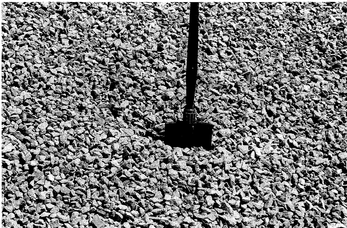
Figure 4. Close up of product pile at Edgewood pit shown in Figure 3. Shovel is approximately 2.5 ft. tall.
