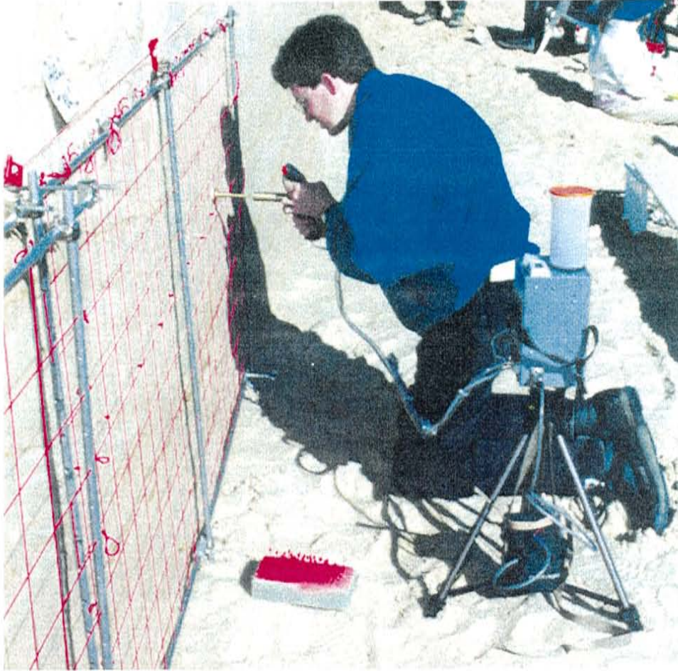
Figure 2.4 — Air permeability measurement taken within a sampling grid on Tier 1.
