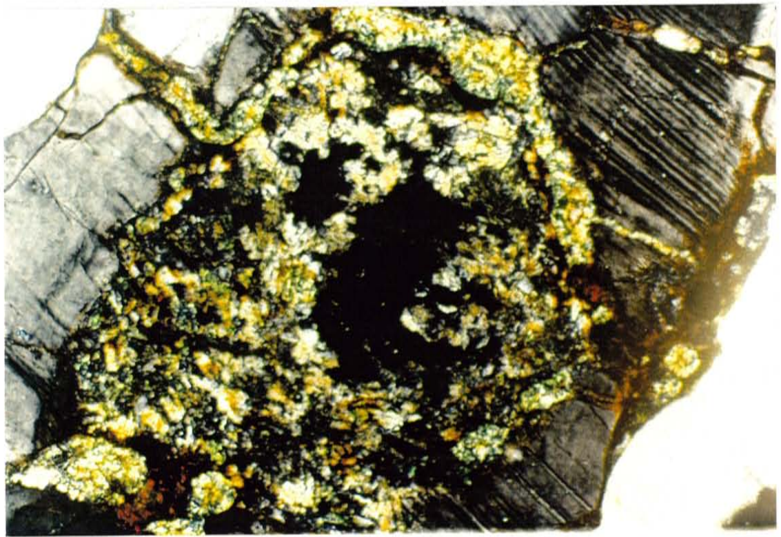
Figure 1.7. Thin section picture (GR-44) of chloritized garnet at 10x (scale=1 mm across). Top: plane polarized light; bottom: crossed polarized light.
