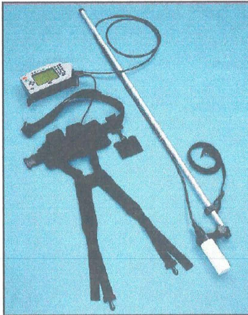
Figure 2.2: The Geometrics G-858 Portable Cesium Magnetometer instrumentation. The G-858 is comprised of a belt-mounted display console connected to a cesium sensor on a hand-held counterbalanced staff. (Geometrics, 1997)
