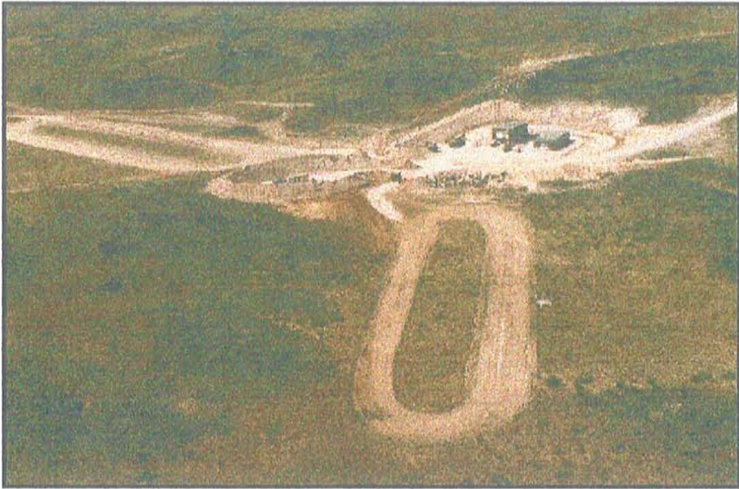
Figure 4.1: Oblique aerial photograph of the EMRTC Counter-Mine Test Site (CTS). The viewed is from the east and shows instrumentation shelters, the Off-Road Track (foreground), and On-Road Track 1 (background). The CTS was developed to test and evaluate technologies for the detection and neutralization of anti-tank mines, anti-personnel mines, and UXO. (EMRTC, 1996)
