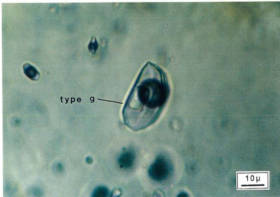
Figure 18. Photomicrograph showing type b, c, and g inclusions in stage 2 quartz.
