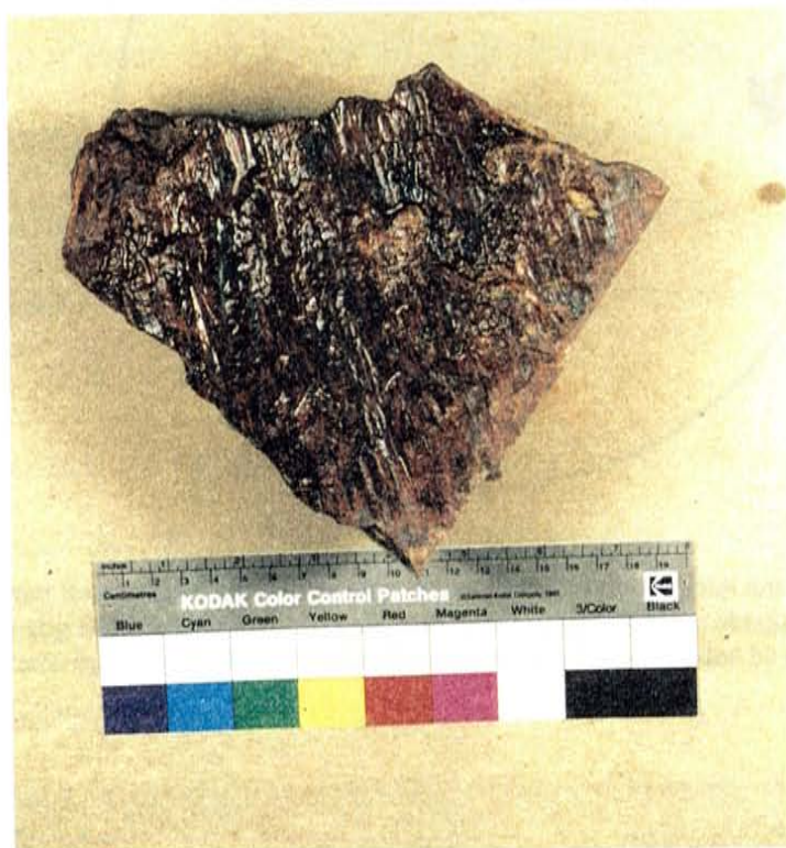
Figure 22. Slickenside striations coated and accentuated by hematite staining from the Coronado fault.
