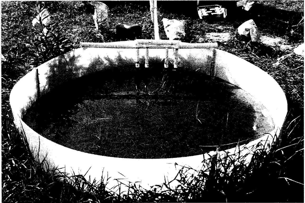
Plate 11. Water supply manifold from site supply tanks to the infiltrometer. Note the live grass in the infiltrometer after two months of constant infiltration, possible only if unsaturated conditions are present.
