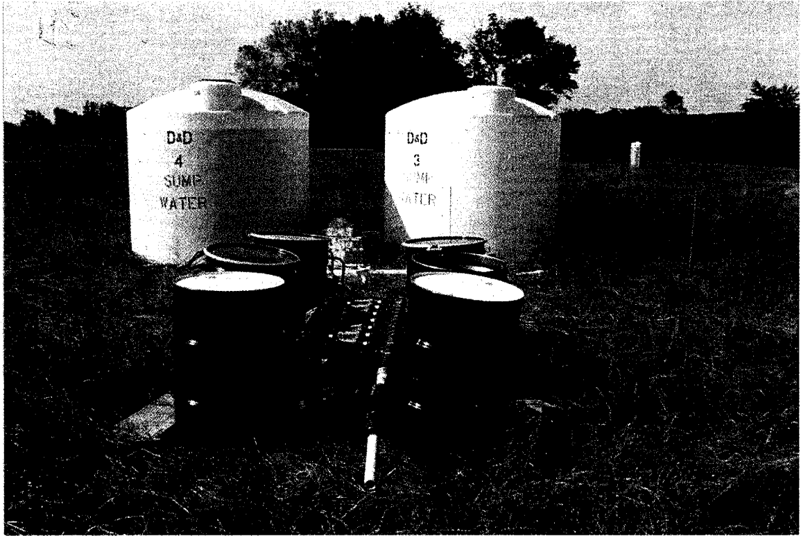
Plate 3. Main supply tanks. The water filter manifold is in the foreground between the two rows of 55 gallon drums.
