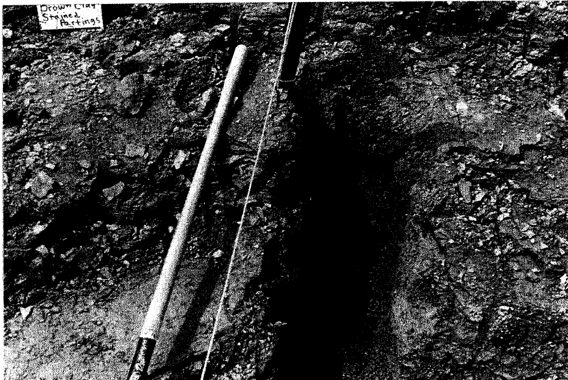
Plate 77. Pink dye (lower right center) can just be seen in the bottom of the trench at sampling site A28-7OL at the far west of the site. The water was moving through a sand stringer originating in the silty sand body in the NW quadrant.
