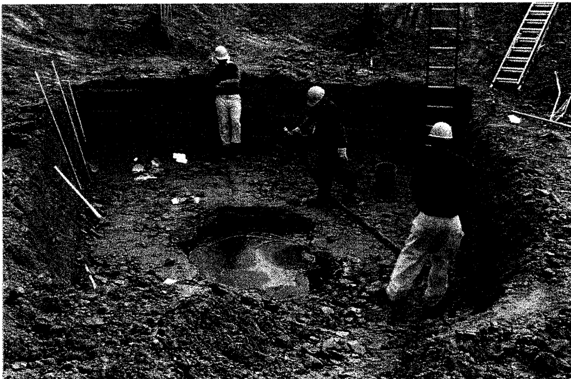
Plate 55 (below). Dye pit at top of Unit 1 (massive unoxidized clays). Depth approximately 3.2 m.
