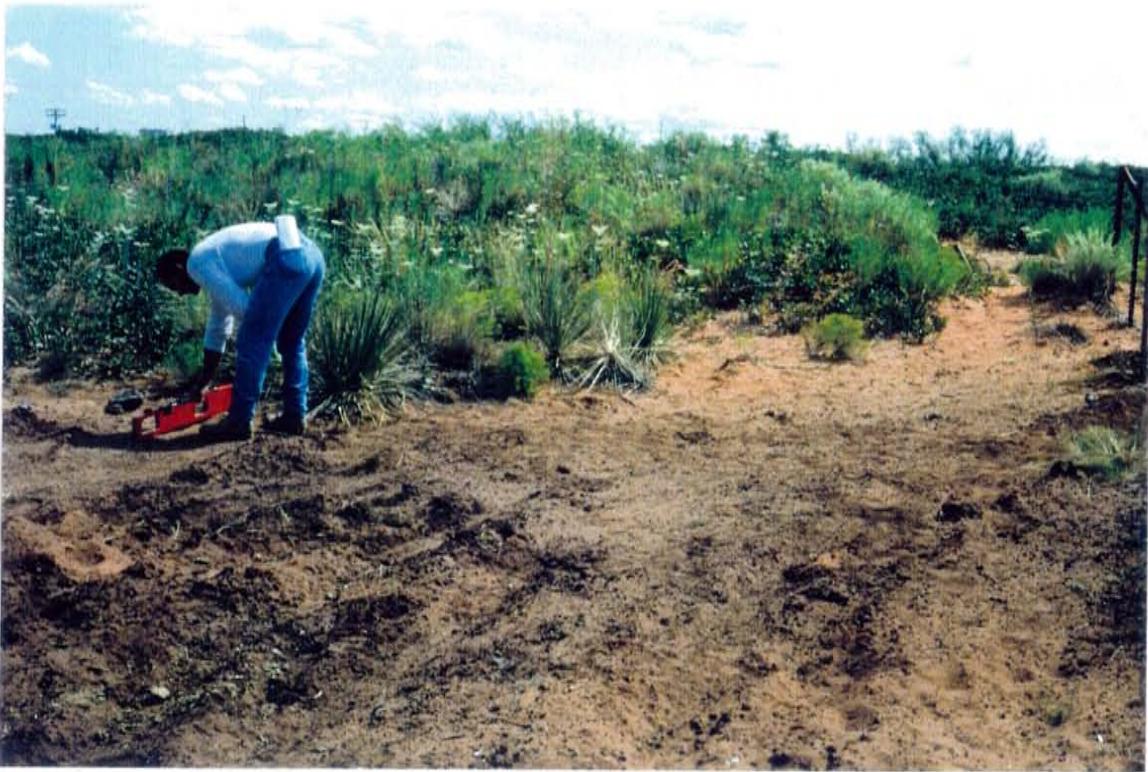
Photo 1. Use of the EM-38 in the vertical mode
