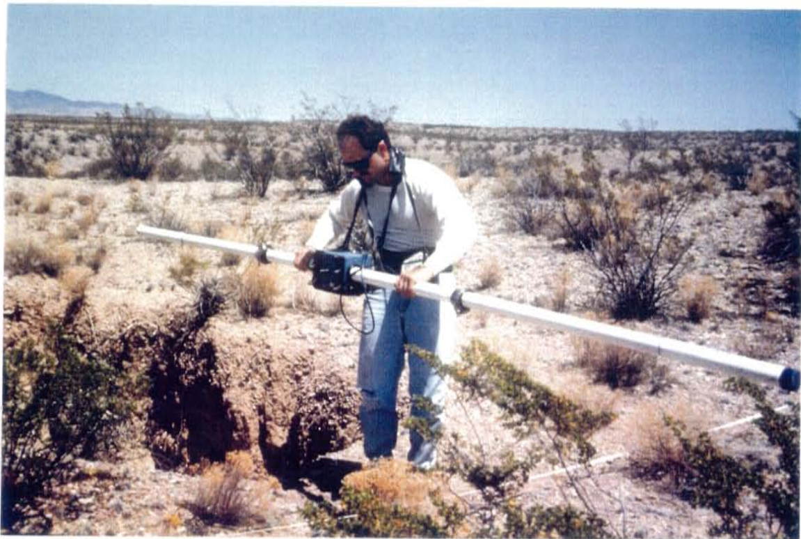
Photo 2. Use of the EM-31 in the horizontal mode (Photo below)
