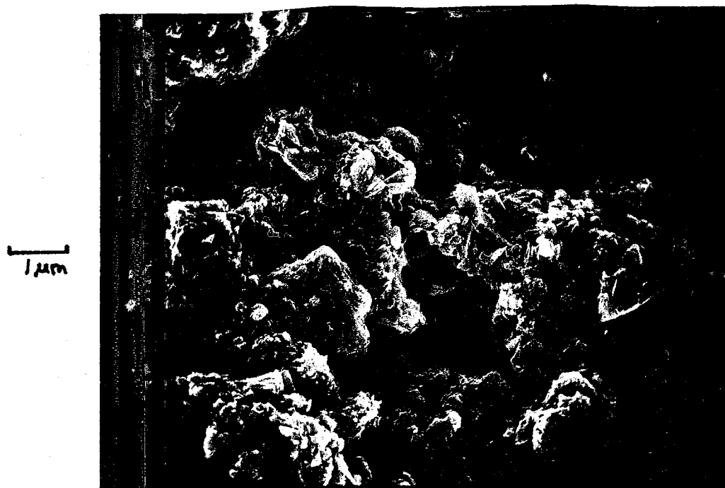
Appendix Figure A2.4. Photomicrograph of HDTMA-modified St. Cloud zeolite with sorbed chromate.
