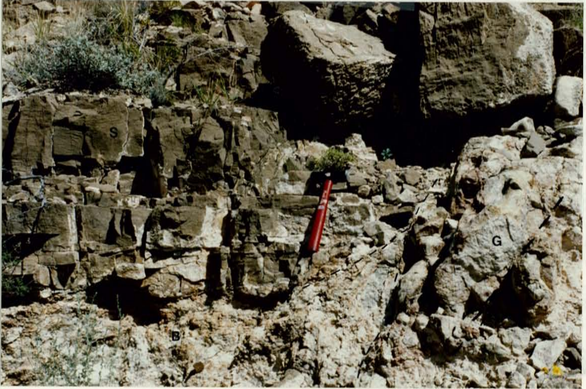
Figure 17. View to the north of gouge zone of Fault 4 cutting low-angle fault between San Andres and Glorieta Formations. S = San Andres Formation; B = Breccia; and G = Gouge. Hammer for scale is 34 cm long.
