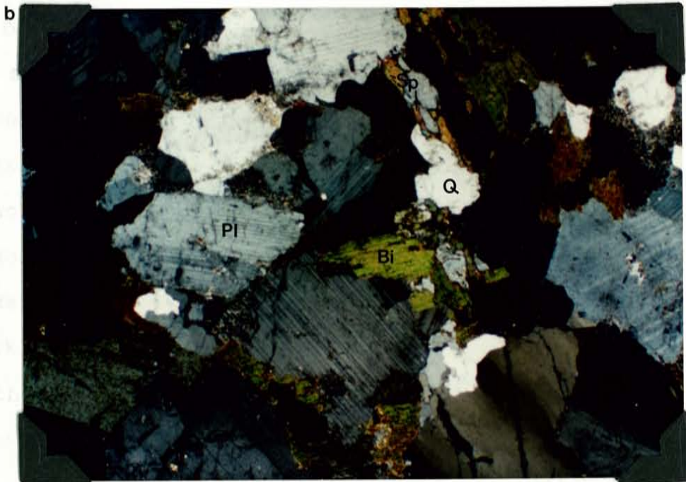
a) Plane light, b) Crossed-nicols. Q=Quartz, Pl=Plagioclase (oligoclase, locally altered to sericite), Mi=Microcline, Bi=Biotite, Op=Opagues (ilmenite, magnetite), Sp=Sphene.
