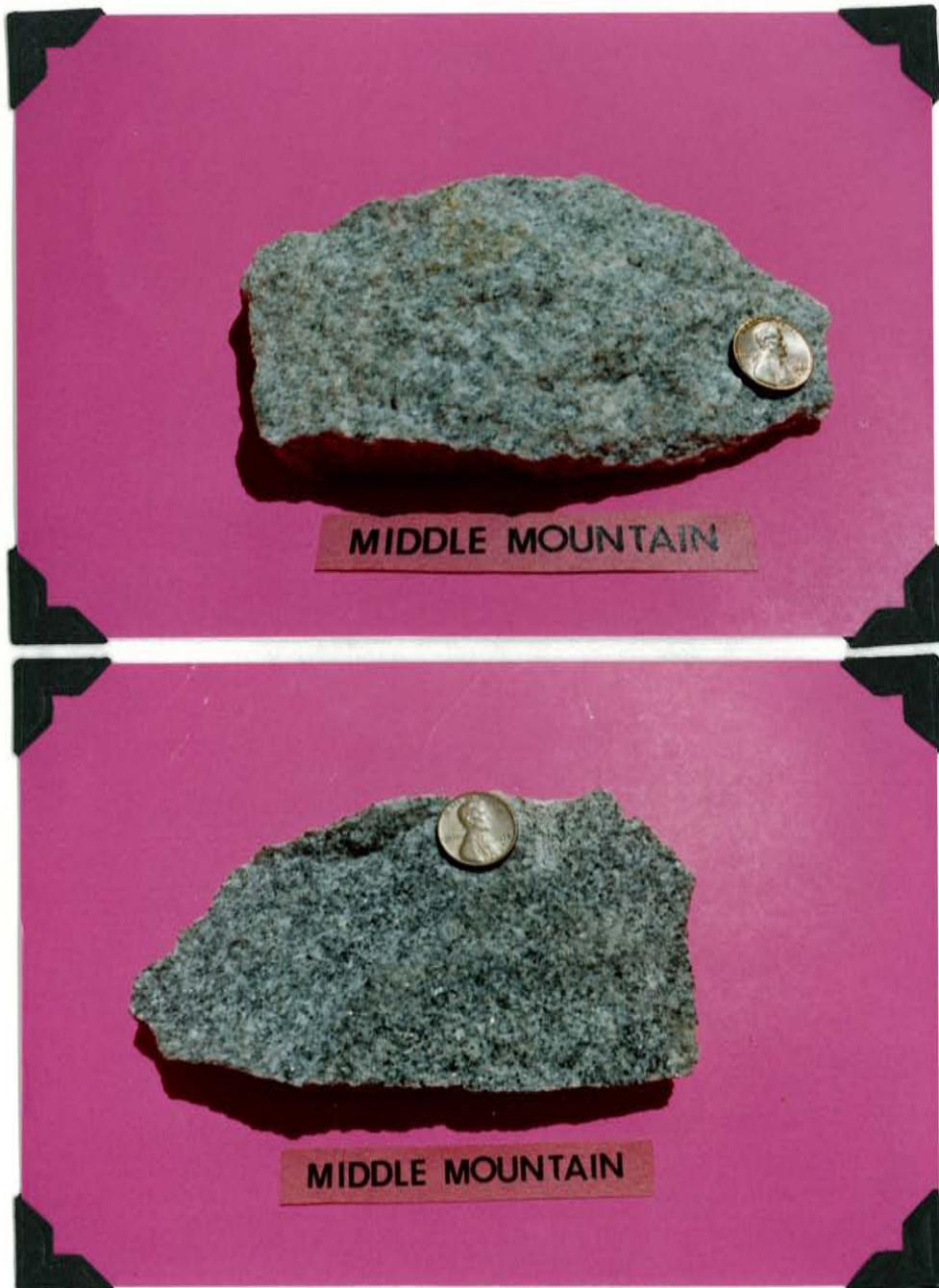
Middle Mountain pluton: a) A grey to pale pink biotite granite, containing scattered randomly oriented microcline megacrysts (.5-1cm long) in a groundmass of plagioclase, quartz, microcline, and biotite. b) a more equigranular grey granite of similar composition to (a).
