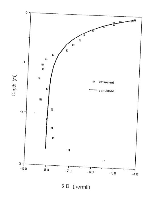
Figure 50 - NIR model calculated versus observed SSIP8  $\delta D$  profile for an isothermal temperature realization
