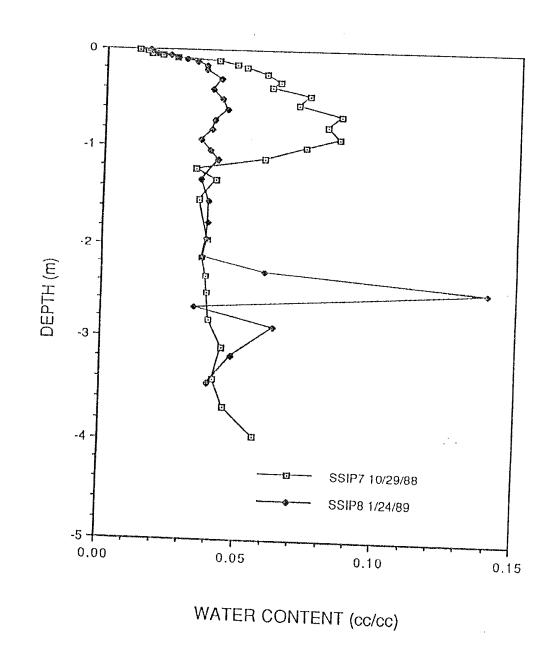
Figure 30 - Depth versus water content for SSIP7 and SSIP8 cores
