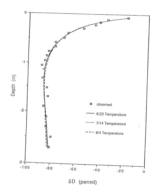
Figure 41 - NIR model calculated versus observed SSIP5  $\delta D$  profile for three simulated temperature realizations
