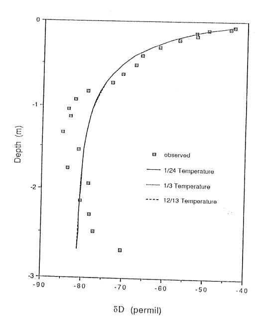
Figure 46 - NIR model calculated versus observed SSIP8  $\delta D$  profile for three simulated temperature realizations
