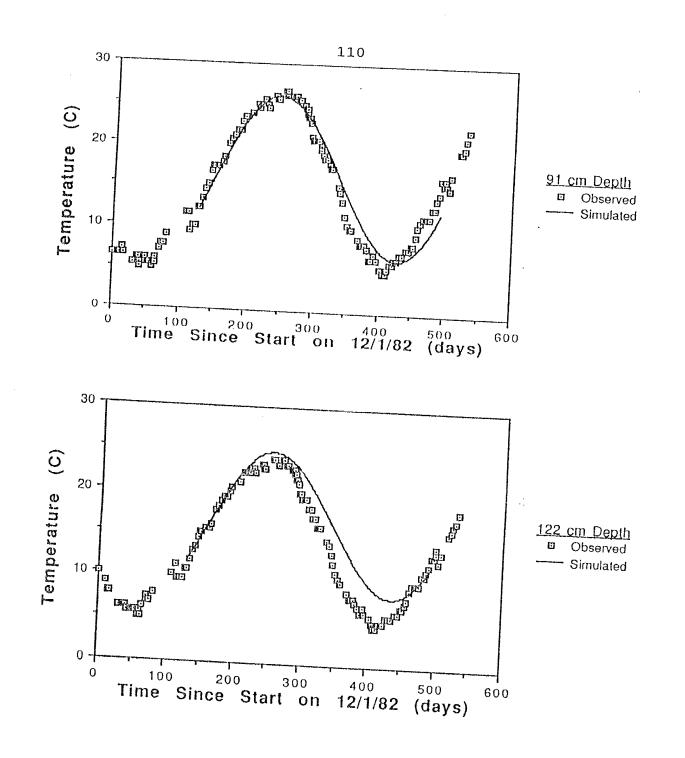
Figure 37 - Results of the analytical heat-flow modeling versus observed temperature data
