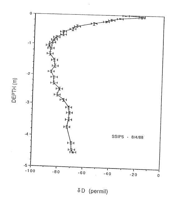
Figure 17 - Depth versus &D for SSIP5 core, Y error bars indicate sampling interval, X error bars indicate 95% confidence interval
