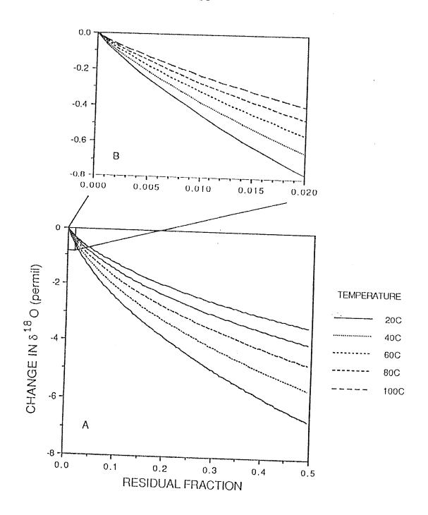
Figure 7 - Change in  $\delta^{18}\text{O}$  versus residual fraction of water remaining during the distillation process. Figure 7B is a subset of 7A
