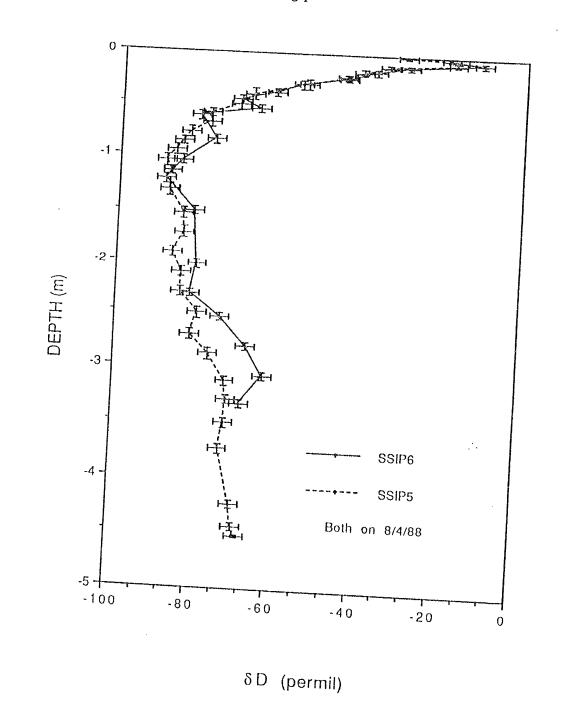
Figure 21 - Depth versus &D for SSIP5 and SSIP6 cores, Y error bars indicate sampling interval, X error bars indicate 95% confidence interval
