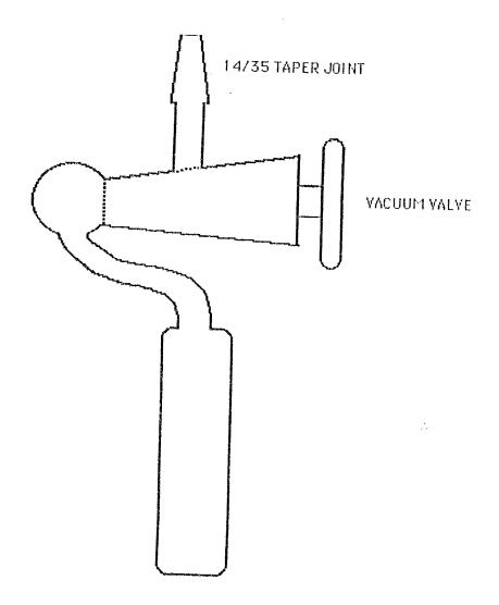
Figure A2 - Schematic of a gas sample bottle
