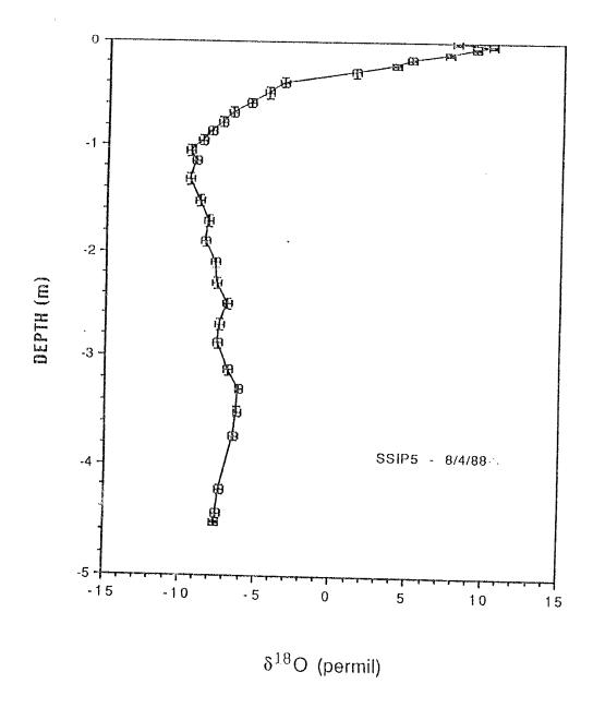
Figure 16 - Depth versus  $\delta^{18}$ O for SSIP5 core, Y error bars indicate sampling interval, X error bars indicate 95% confidence interval
