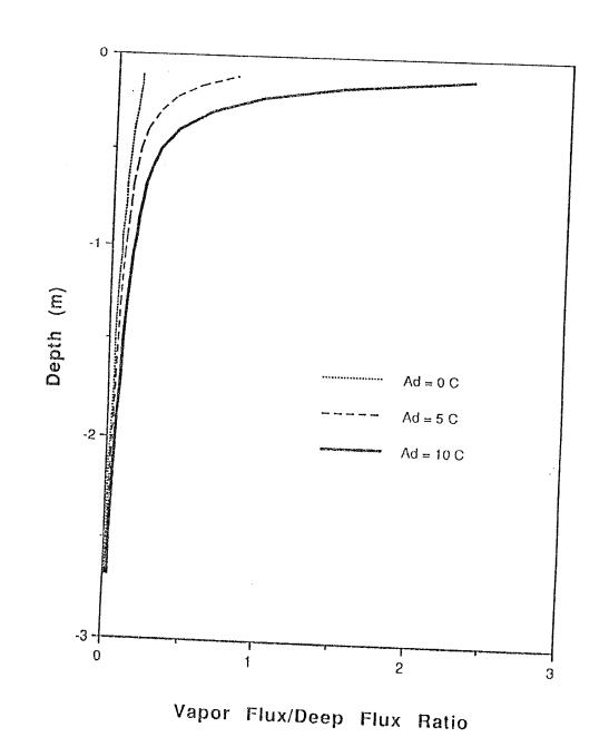
Figure 42 - Simulated vapor flux versus depth for three temperature realizations from SSIP5 data, where A  $_{\delta}$  = 0, 5, and 10°C
