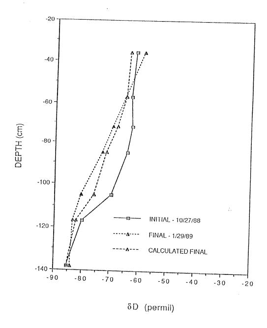
Figure 52 - Depth versus &D for observed data (depth-averaged into seven discrete intervals) and MBM drying model calculated results
