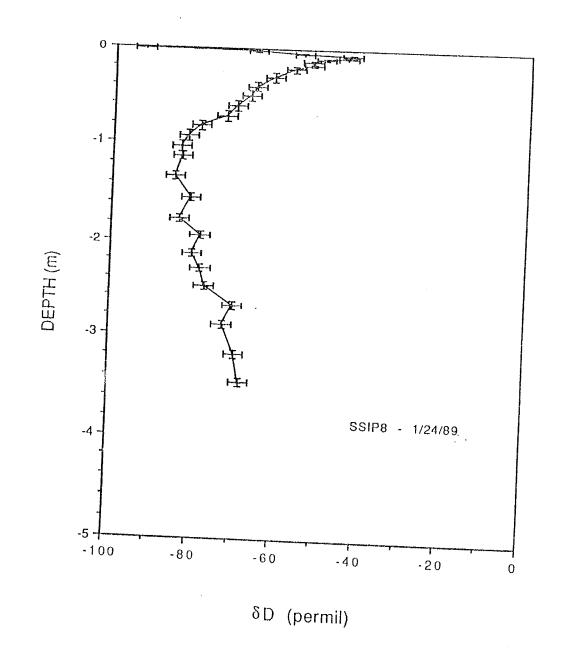
Figure 26 - Depth versus  $\delta D$  for SSIP8 core, Y error bars indicate sampling interval, X error bars indicate 95% confidence interval
