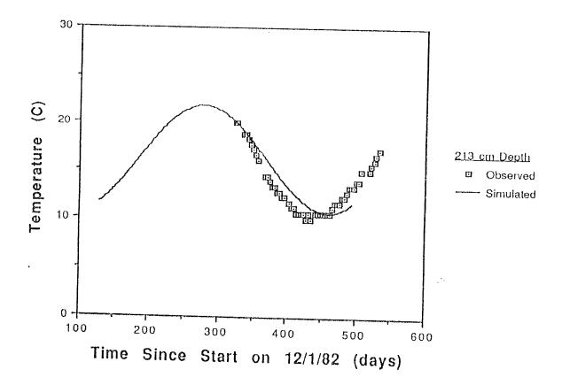
Figure 39 - Results of the analytical heat-flow modeling versus observed temperature data
