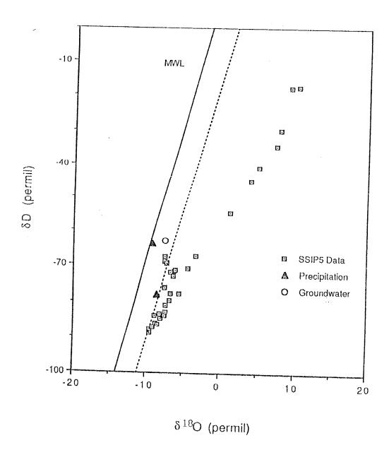
Figure 54 -  $\delta D$  versus  $\delta^{18}O$  for the SSIP5 core, with the MWL, and a line drawn parallel to the MWL at the intersection of the SSIP5 data to determine the deuterium excess for the PD/M recharge model
