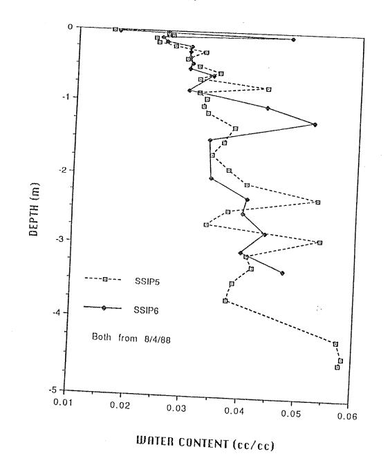
Figure 20 - Depth versus water content for SSIP5 and SSIP6
