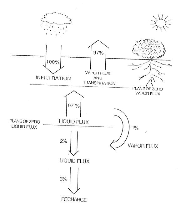
Figure 45 - Conceptual depiction of soil-moisture movement under summer conditions. The plane of zero vapor flux occurs approximately 0.07 m below land surface, and the plane of zero liquid flux at 0.35 m.
