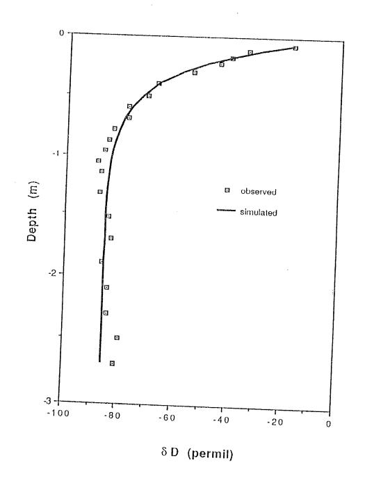
Figure 49 - NIR model calculated versus observed SSIP5  $\delta D$  profile for an isothermal temperature realization
