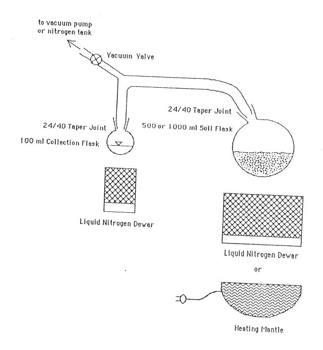
Figure 5 - Schematic diagram of vacuum distillation line setup
