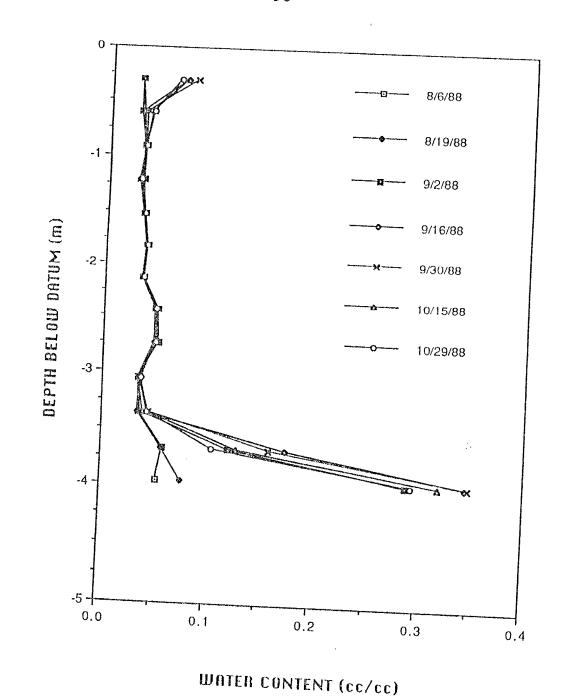
Figure 32 - Depth versus water content data from neutron logging for various times at the Stephens, Hicks, and Stein site (Stein, T. written communication, March 1989)
