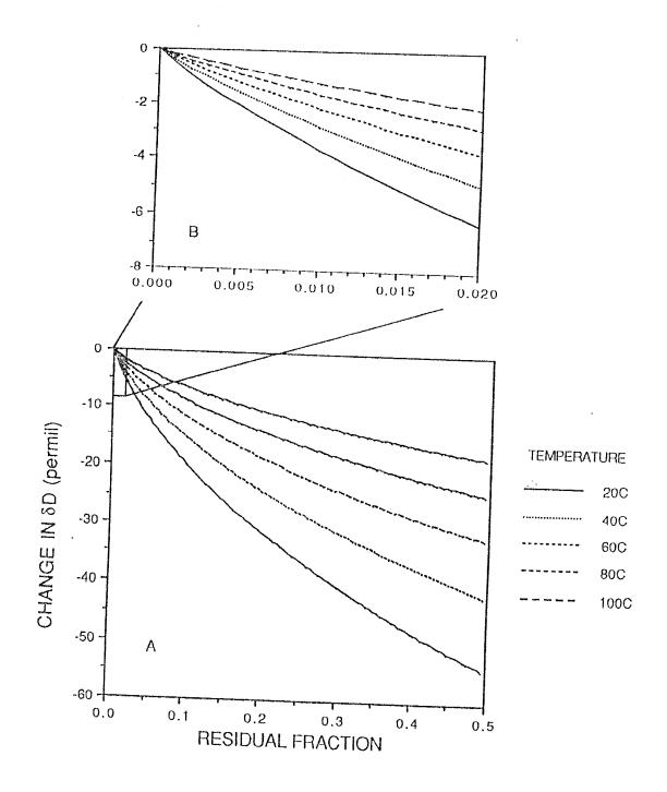
Figure 6 - Change in  $\delta D$  versus residual fraction of water remaining during the distillation process. Figure 6B is a subset of 6A
