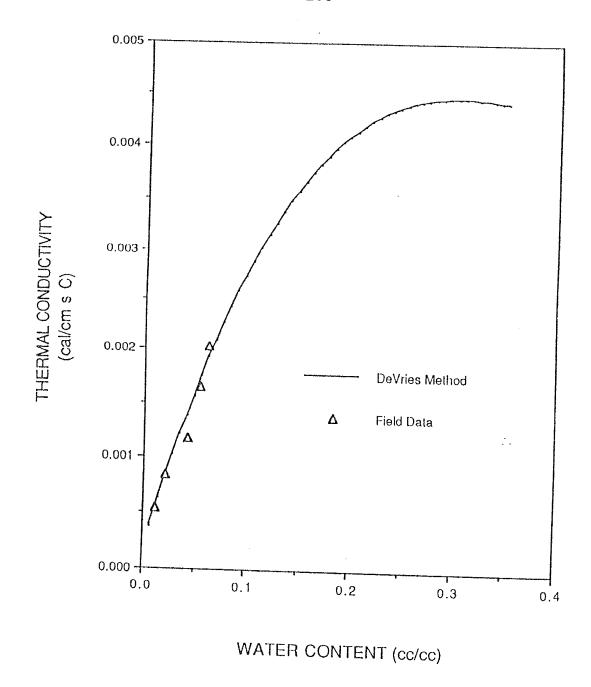
Figure 34 - Thermal conductivity versus water content data, data points from in-situ experimental results, calculated functional relationship from DeVries (1963) method
