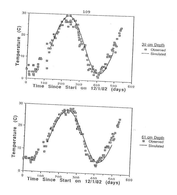
Figure 36 - Results of the analytical heat-flow modeling versus observed temperature data
