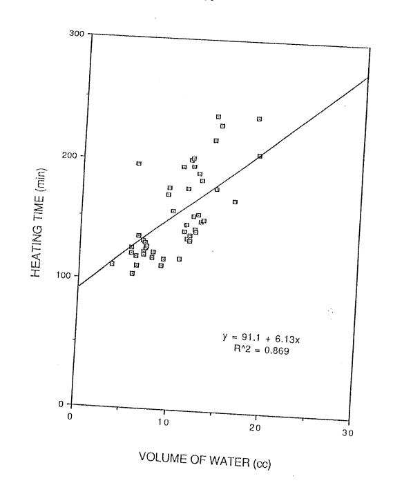
Figure 10 - Heating time versus volume of soil water distilled from field samples collected by Knowlton et al. (1989)
