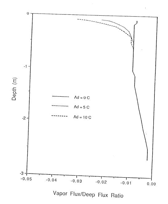
Figure 47 - Simulated vapor flux versus depth for three temperature realizations from SSIP8 data, where  $A_{\delta}=0$ , 5, and 10°C
