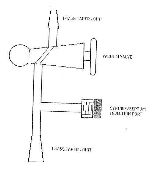
Figure A4 - Schematic of the  ${\rm H}_{\rm 2}$  reduction reaction vessel
