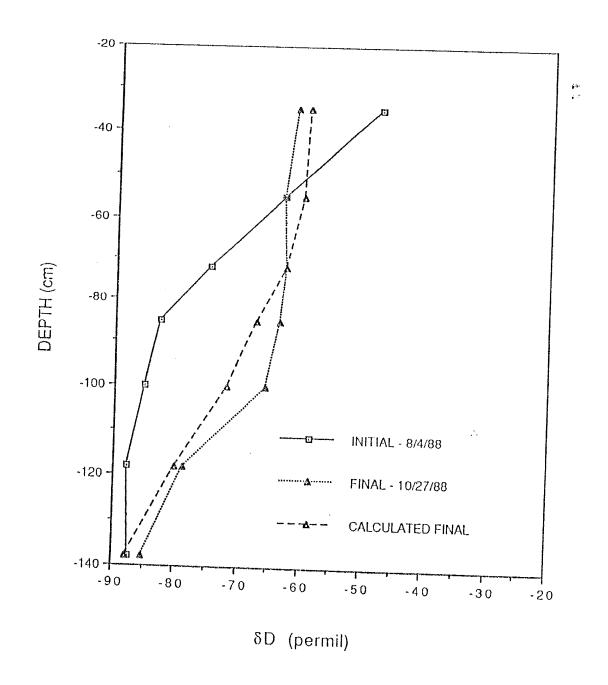
Figure 51 - Depth versus  $\delta D$  for observed data (depth-averaged into seven discrete intervals) and MBM wetting model calculated results
