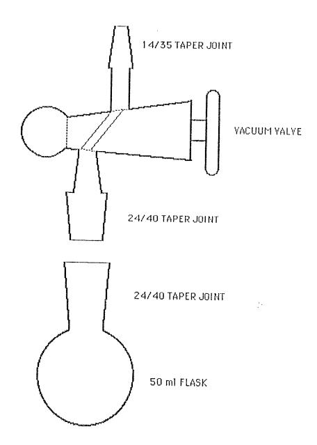
Figure A3 - Schematic of the  ${\rm CO_2/H_2O}$  reaction vessel
