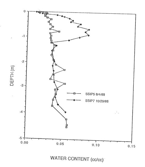
Figure 23 - Depth versus water content for SSIP5 and SSIP7 cores
