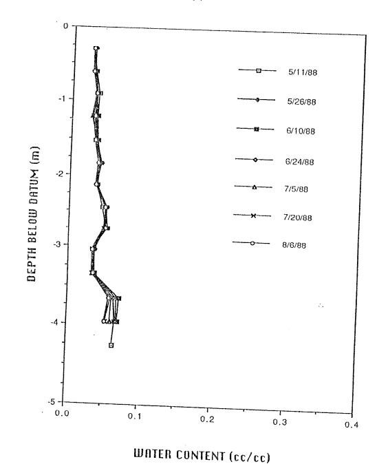
Figure 31 - Depth versus water content data from neutron logging for various times at the Stephens, Hicks, and Stein site (Stein, T. written communication, March 1989)
