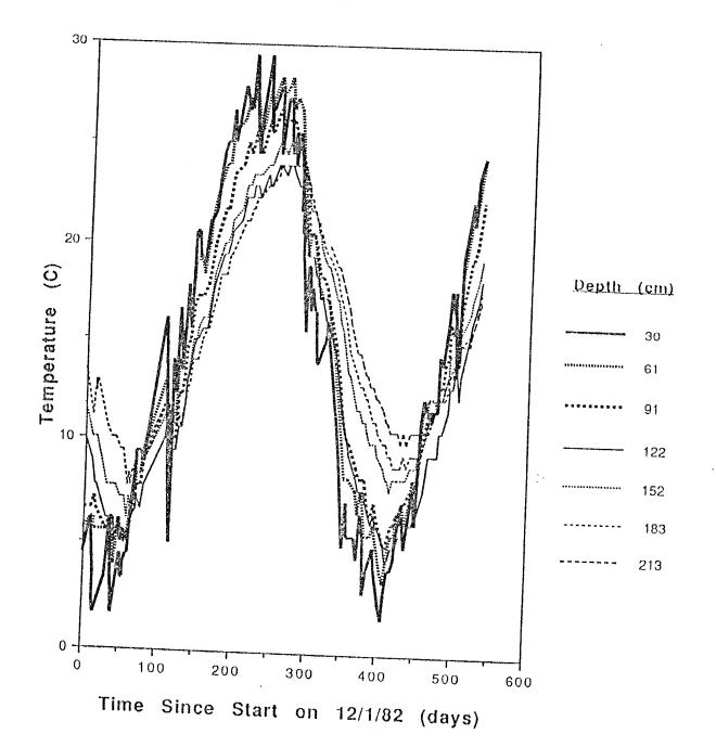
Figure 35 - Observed temperature versus time for seven depths between 30 and 210 cm, starting 12/1/82 (from Stephens et al., 1985)
