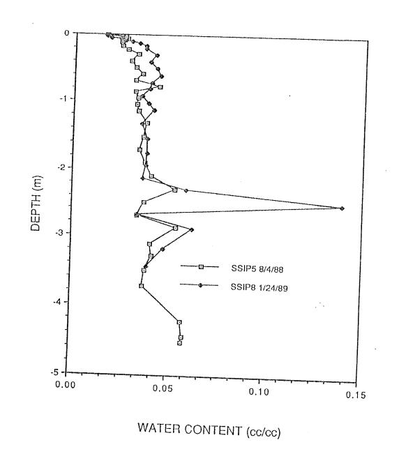
Figure 29 - Depth versus water content for SSIP5 and SSIP8 cores
