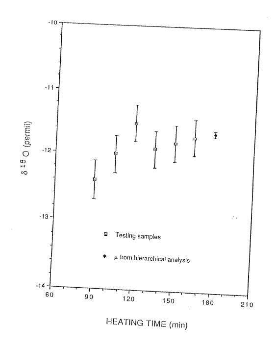
Figure 9 -  $\delta^{18}$ O versus heating time for a sand with 15 ml of water, and volumetric water content of 0.115 cc/cc. The mean and 95% confidence intervals are calculated from the hierarchical statistical analysis
