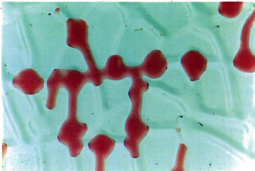
Figure 60. Photomicrograph of a complex blob observed in the micromodel.
