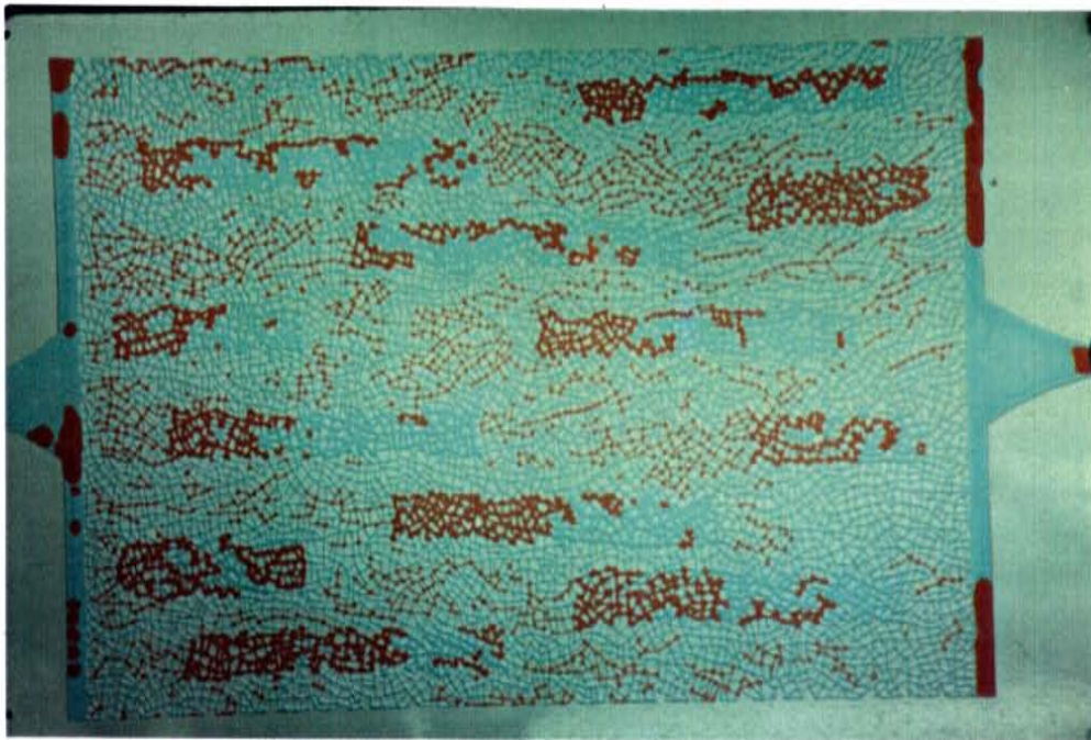
Figure 74. Lens model, run at fast rate, at residual saturation.
