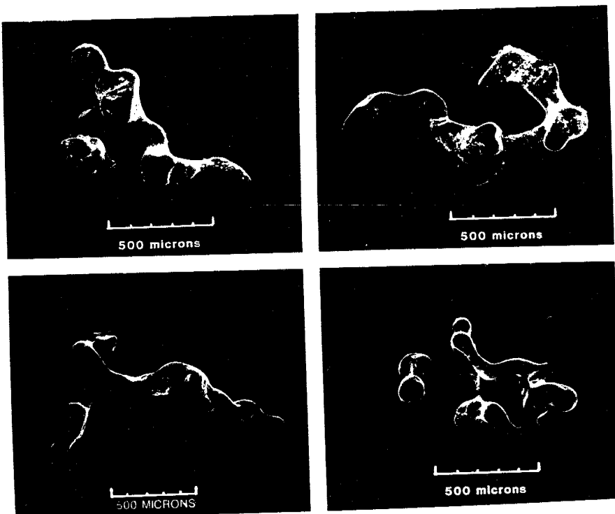
Figure 64. SEM photomicrographs of branched blob casts from Sevilleta sand column.
