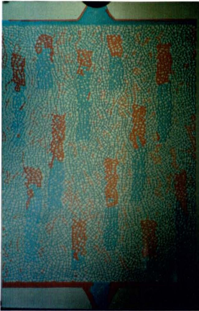
Figure 75. Lens model, vertically held run at slow rate at residual saturation.
