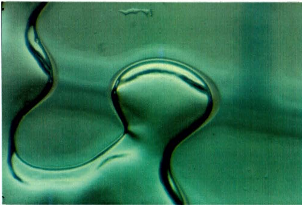
Figure 91. Detail a thin organic liquid film located between the gas and water. The photo represents steady state conditions after the Soltrol has been drained by air from the vadose zone model.
