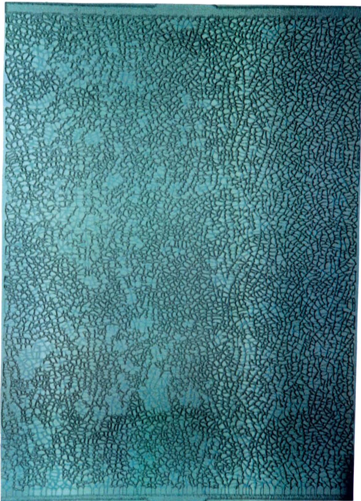
Figure 86. Initial vadoso zone condition, with water drained by air to residual (irreducible) water saturation. The water was dyed blue, and the air was not dyed.
