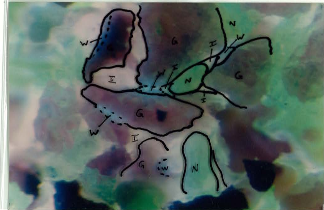
Figure 15. Photomicrograph of three-phase system. On the overlay 'w' stands for wetting phase, 'I' stands for intermediate wetting, 'N' stands for the non-wetting phase, and 'G' stands for grain. Note the well drained pore. Sample is magnified 100 times
