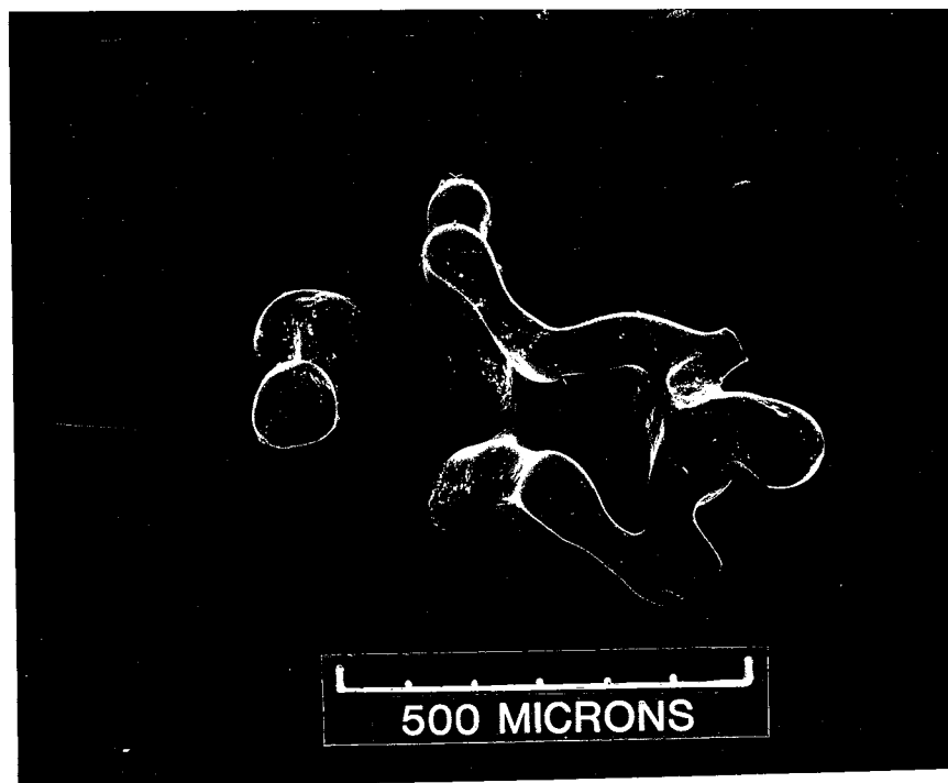
Figure 2-12. Complex shaped organic liquid possibly trapped by by-passing (Peplinski, 1989).
