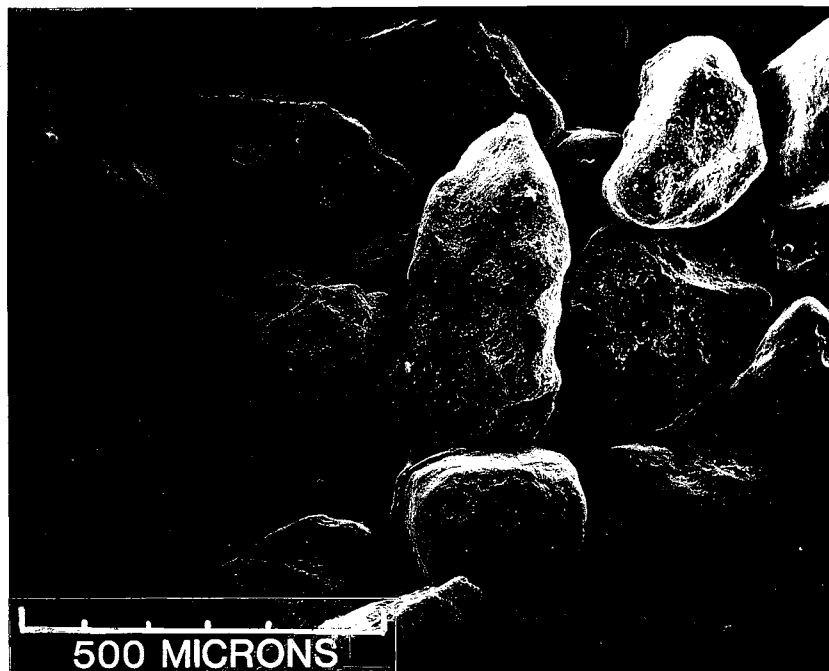
FIGURE 4-2. SEM photomicrograph of Sevilleta sand (From Wilson et al., 1989)
