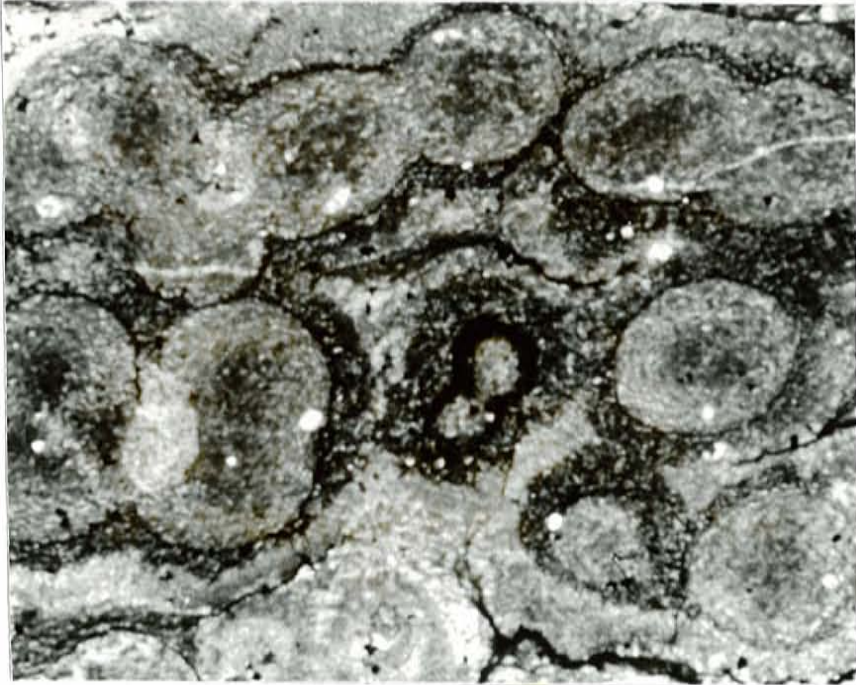
Figure 5. Photomicrograph of oolitic ferruginous chert. Plane-polarized light, 5x, width of photo covers 6.5 mm.
