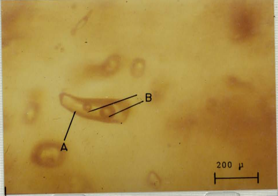
Figure 46. "Double-bubbles" T = + 2.6 C (The smaller bubble homogenized at +8.8 C while the larger increased in size). 110-35-24 quartz from a vug in the en echelon shears.
