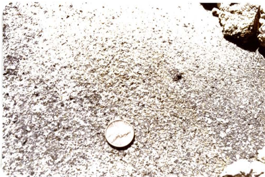
Fig. 5. Burrego Formation: Unit 2; biosparite / grainstone. Coin = 1.9 cm.
