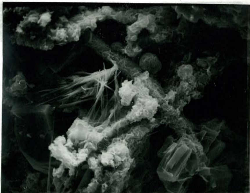
Plate 23. Crenulated montmorillonite covering glass shards. 10 \mu m , Sample 13-1; Magnified 1000X.
