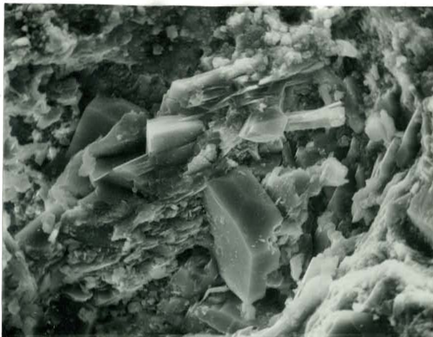
Plate 35. Well developed crystal terminations on 10.5 μm authigenic potassium feldspar prisms. Sample 13-19; Magnified 900X.
