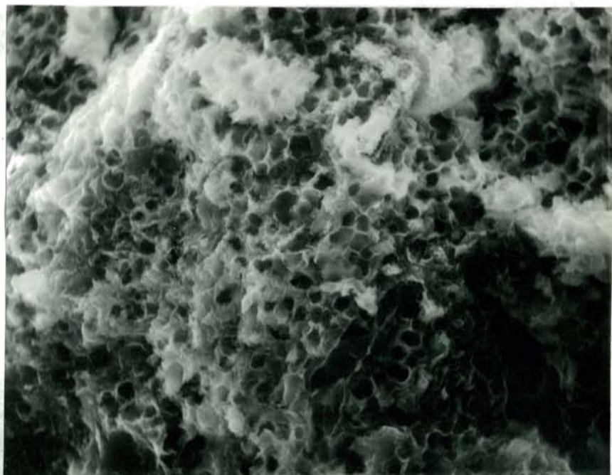
Plate 24. Honeycomb montmorillonite habit. 7.5 \mu m , Sample 13-9; Magnified 1500X.
