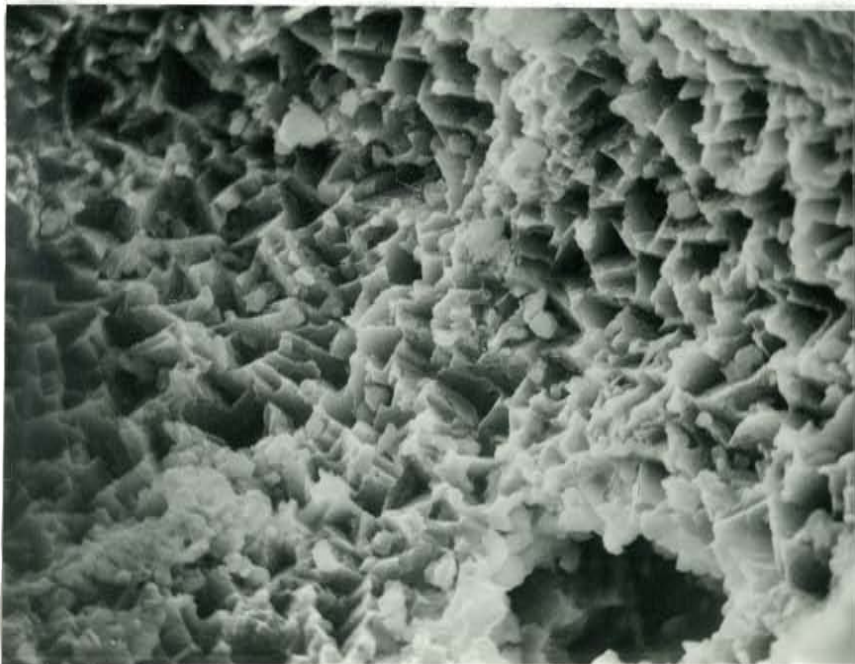
Plate 25. Interlocking montmorillonite crystals pervasively cover glassy surfaces. 9.0 \mu m Sample 30-18; Magnified 1200X.
