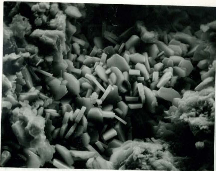
Plate 29. Wafer-thin, coffin-shaped, heulandite group zeolite laths. 10 \mu m Sample 30-20; Magnified 1000X.
