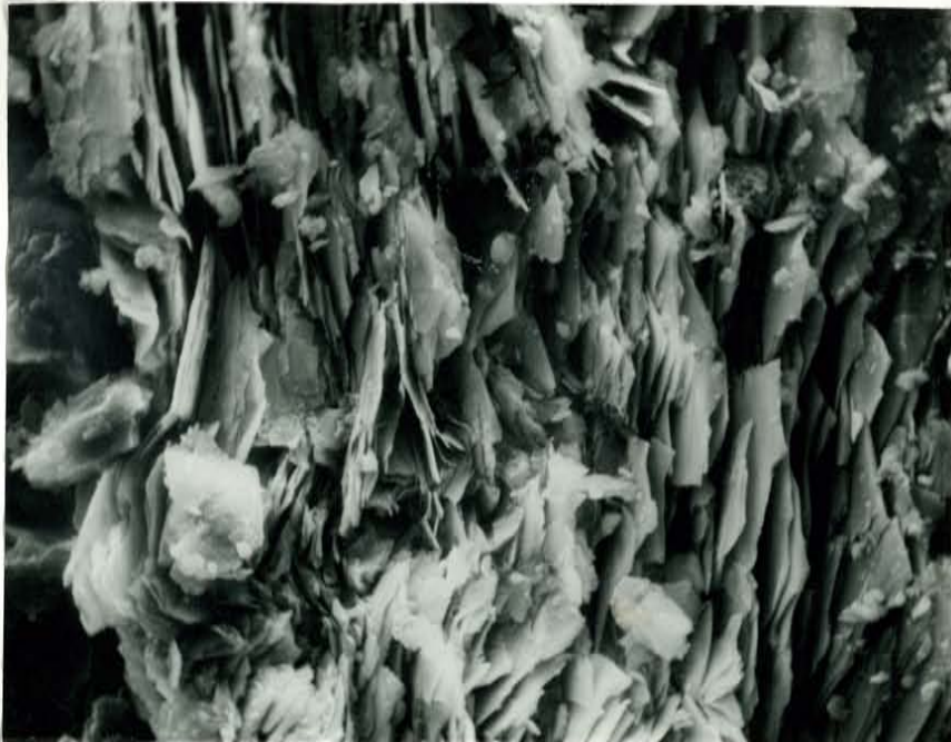
Plate 21. Authigenic illite showing micaceous habit. 10 \mu m Sample 30-9; Magnified 1000X
